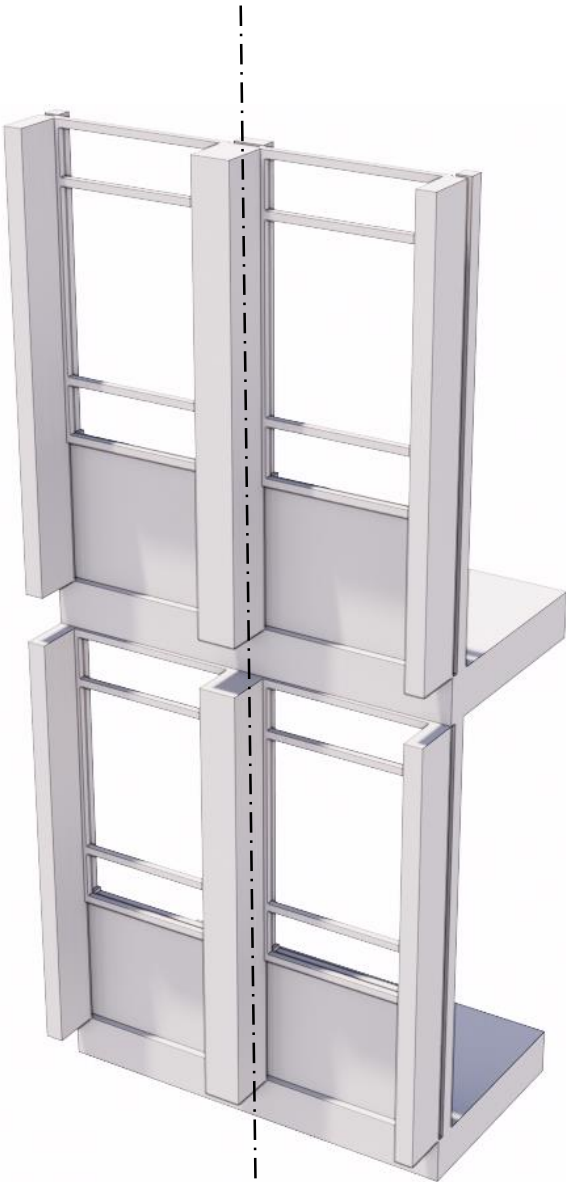
Structural Grid Line
