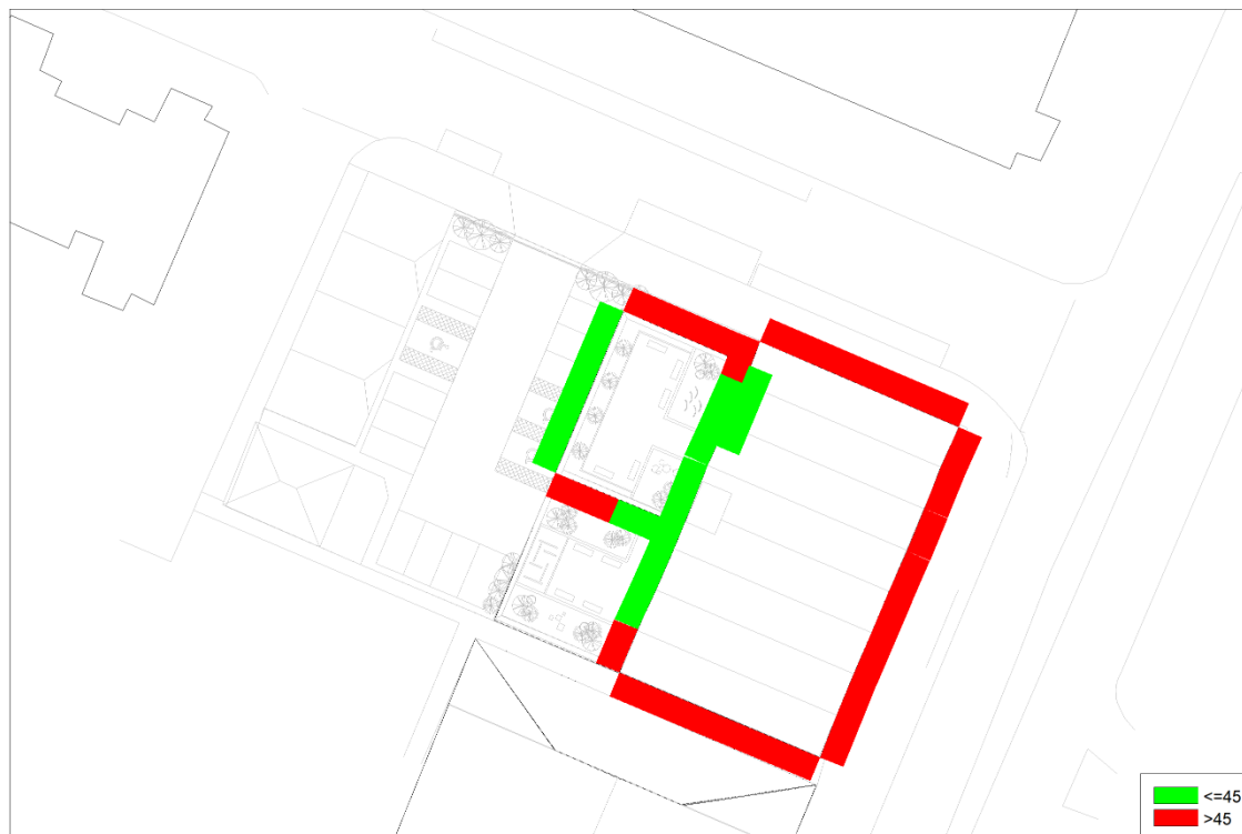
Figure 5: Night-Time Façade Noise Levels (dB LAeq,8h (free-field))
