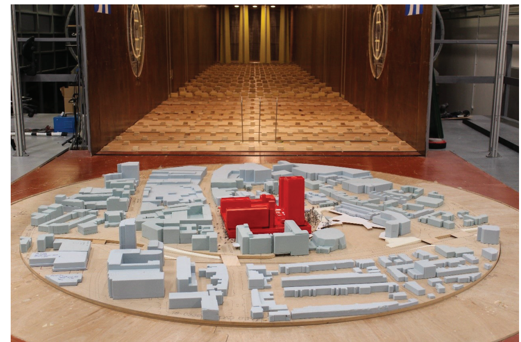
Figure 10.29 Proposed Development with Existing Surrounding Buildings (Configuration 2) – View in the Wind Tunnel (from the west)
