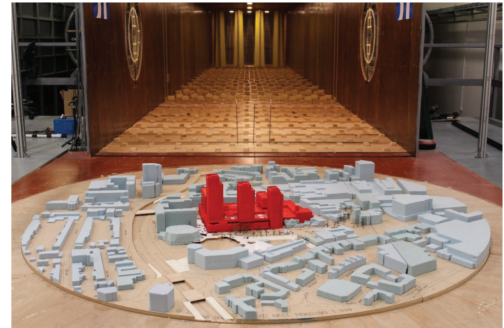
Figure 10.28 Proposed Development with Existing Surrounding Buildings (Configuration 2) – View in the Wind Tunnel (from the south)
