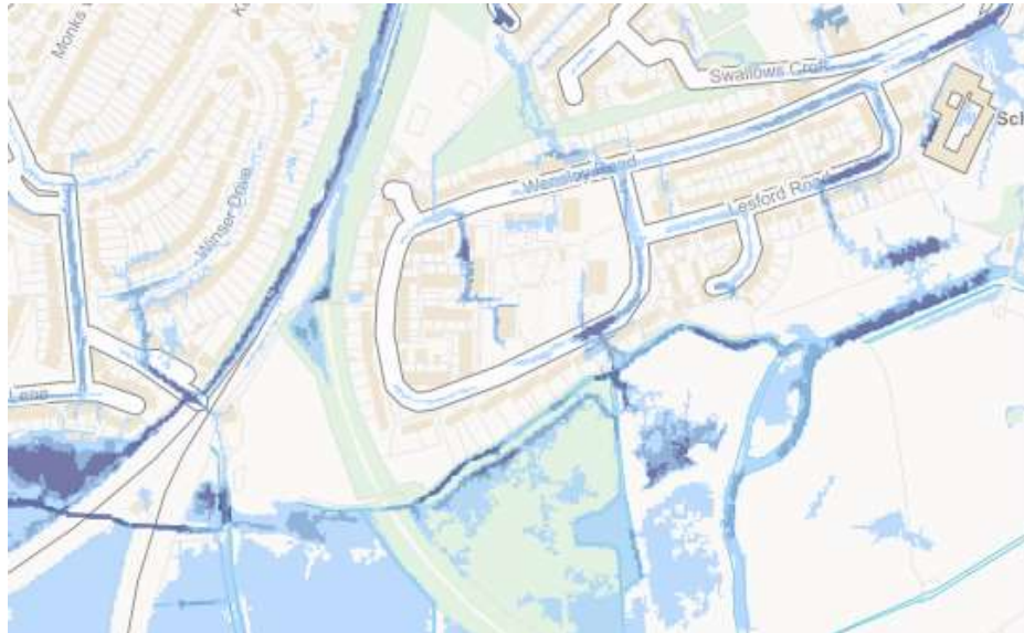
Figure 7.5 Surface Water Flood Risk map
