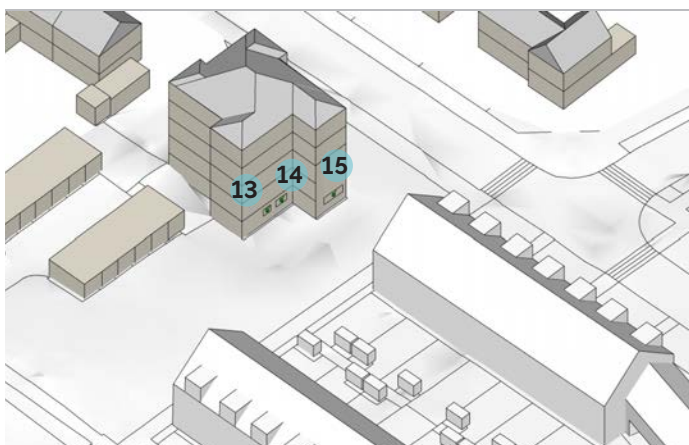
Figure 17. Labelled windows for VSC analysis
