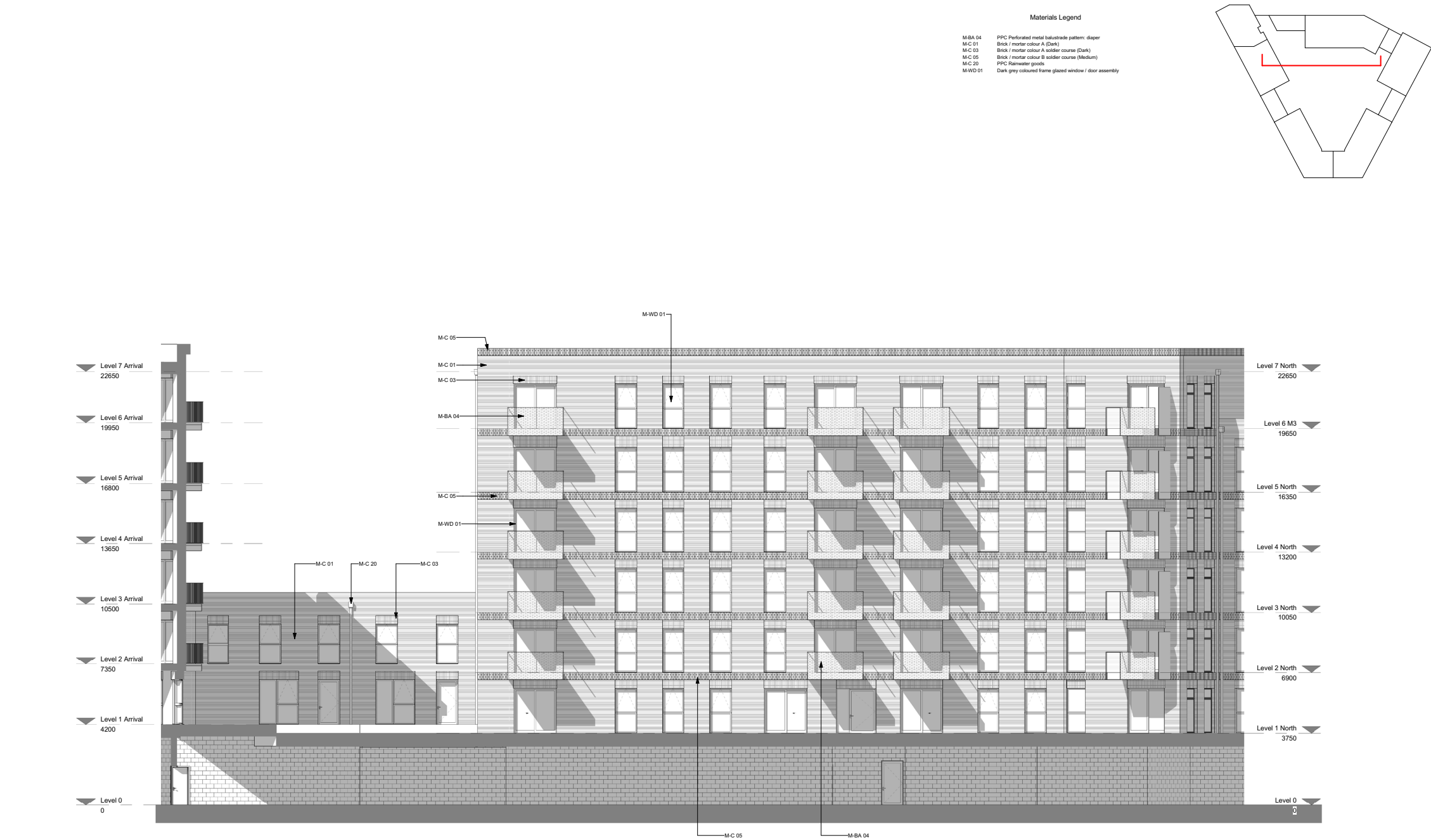
Middle Block Courtyard South Elevation 1 : 100
