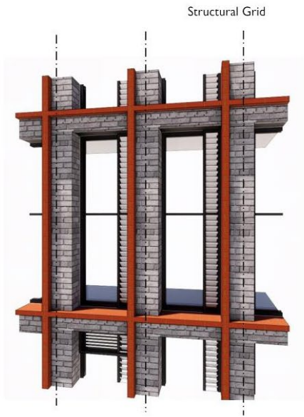
Facade Type 1 - Brickwork
