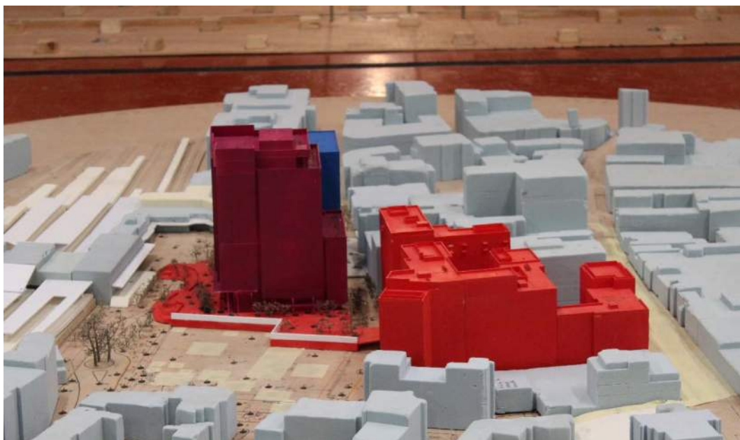
Figure 42: Interim Development Scenario with Landscaping, Wind Mitigation and the Existing Surrounding Buildings – View in the Wind Tunnel (from the west)
