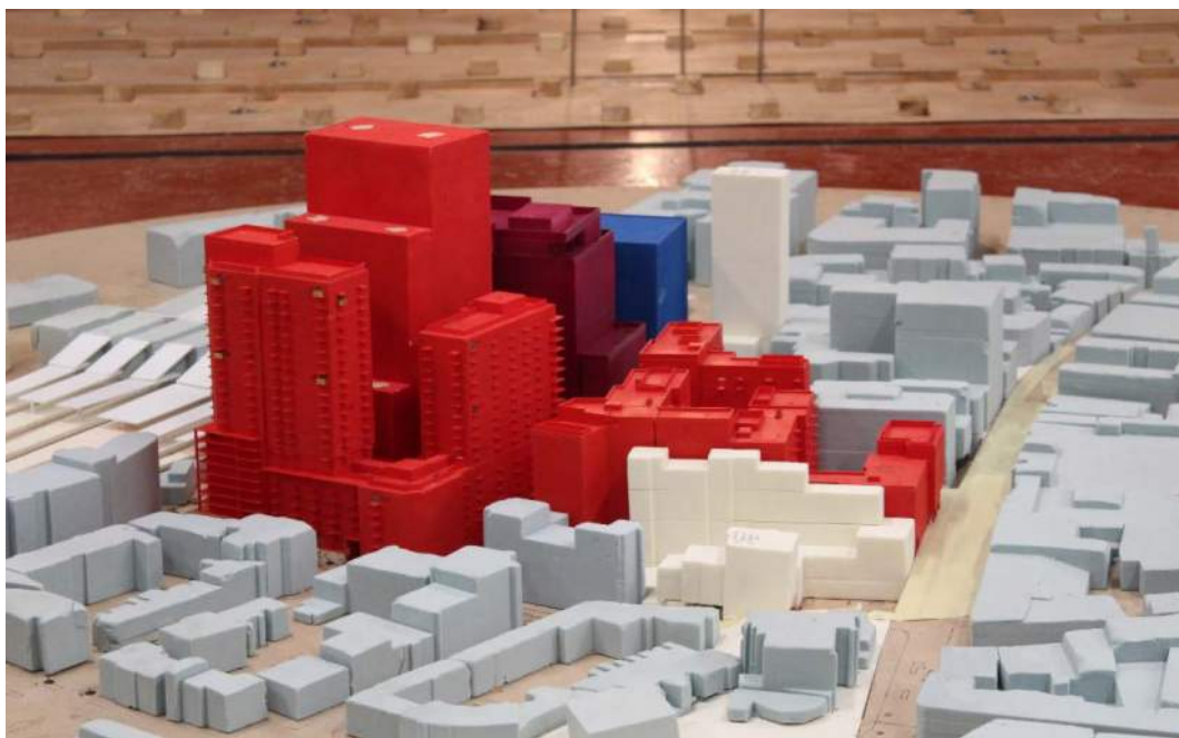
Figure 44: Development Option 1 with Landscaping, Wind Mitigation and the Cumulative Surrounding Buildings – View in the Wind Tunnel (from the south-west)
