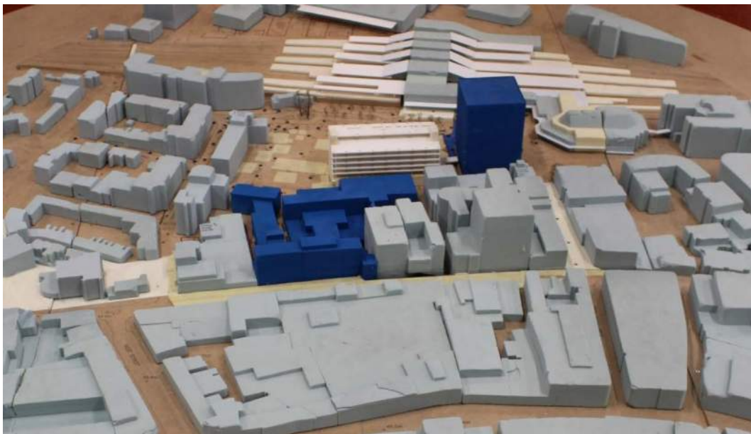
Figure 34: Existing Site with the Existing Surrounding Buildings – View in the Wind Tunnel (from the south)
