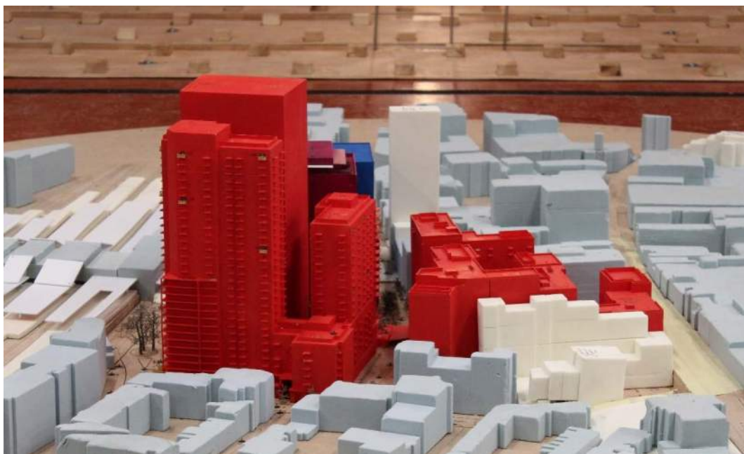
Figure 46: Development Option 2 with Landscaping, Wind Mitigation and the Cumulative Surrounding Buildings – View in the Wind Tunnel (from the south-west)
