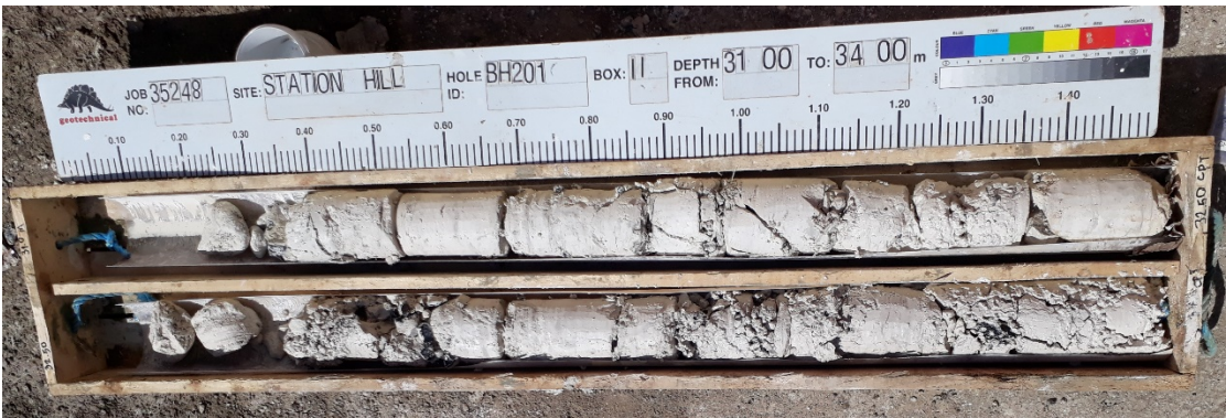
Photograph 3: Structured Chalk in BH201 (Source: GEL Factual Report 35248)
