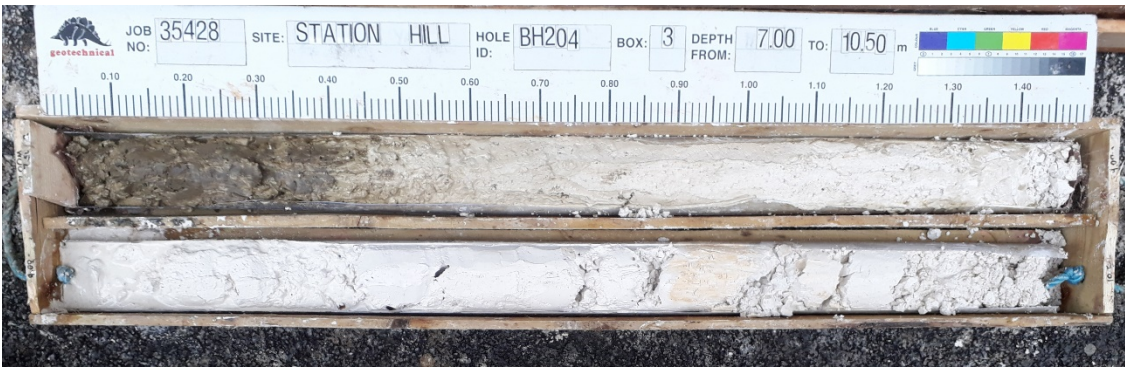
Photograph 2: Structureless Chalk in BH204 (Source: GEL Factual Report 35248)
