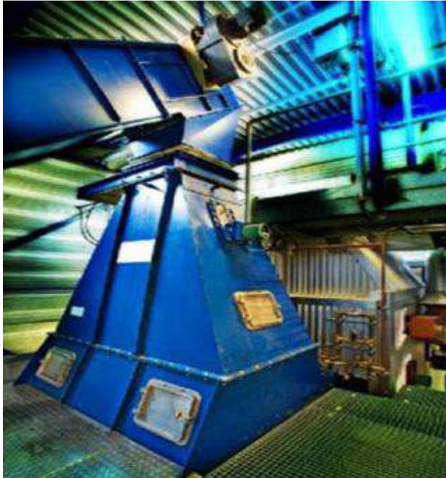
Figure 8: Material in-feeder unit
