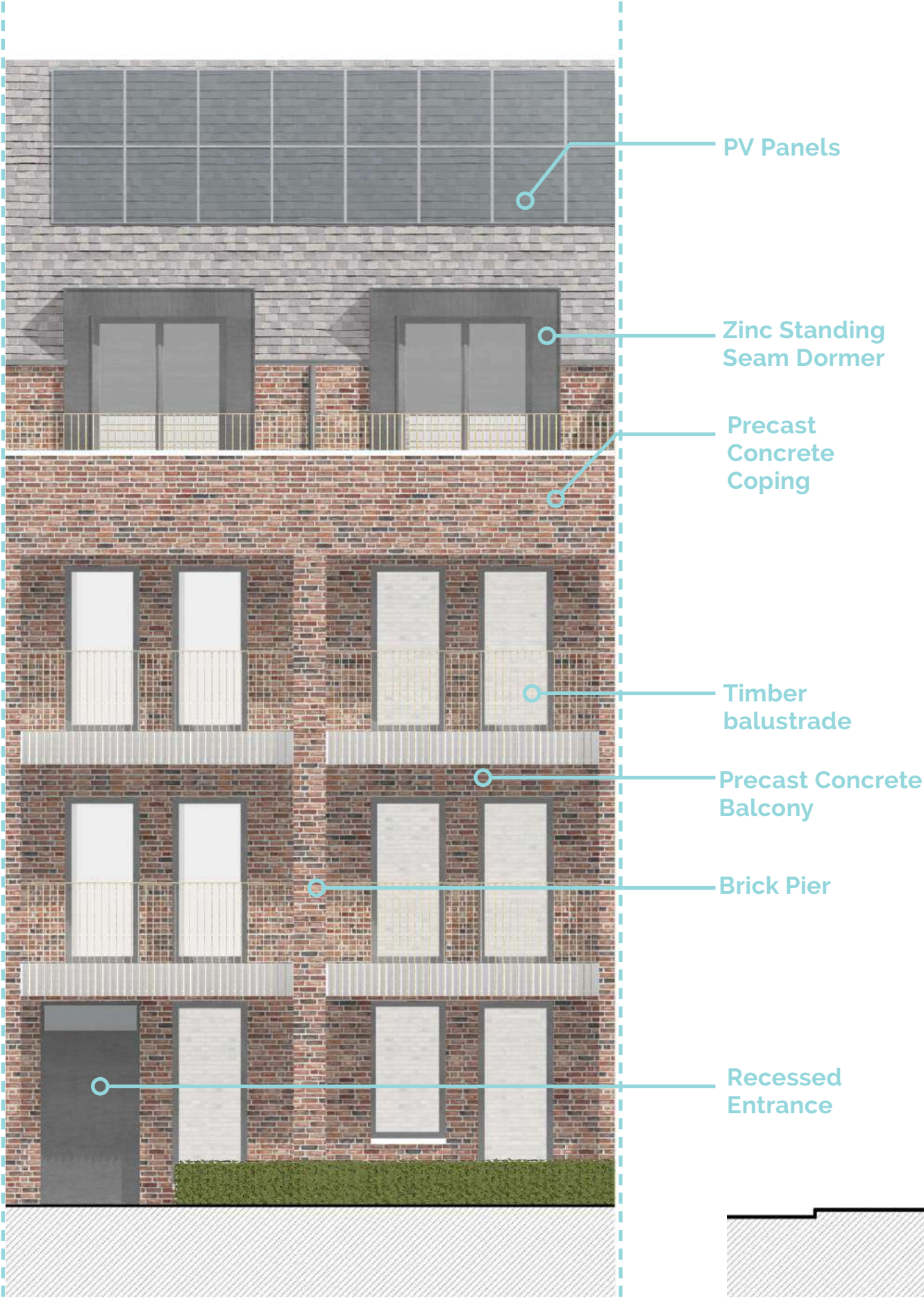
Elevation Study - Apartment Building South Elevation
