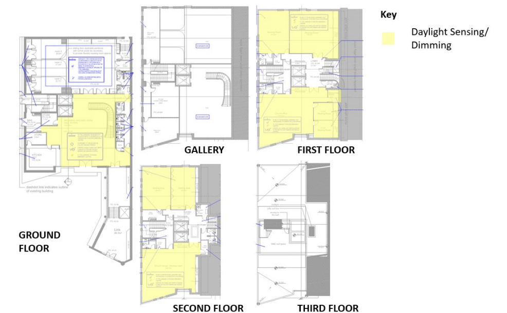
Figure 7: Proposed Greyfriars Centre Daylight Sensing Controls Strategy
