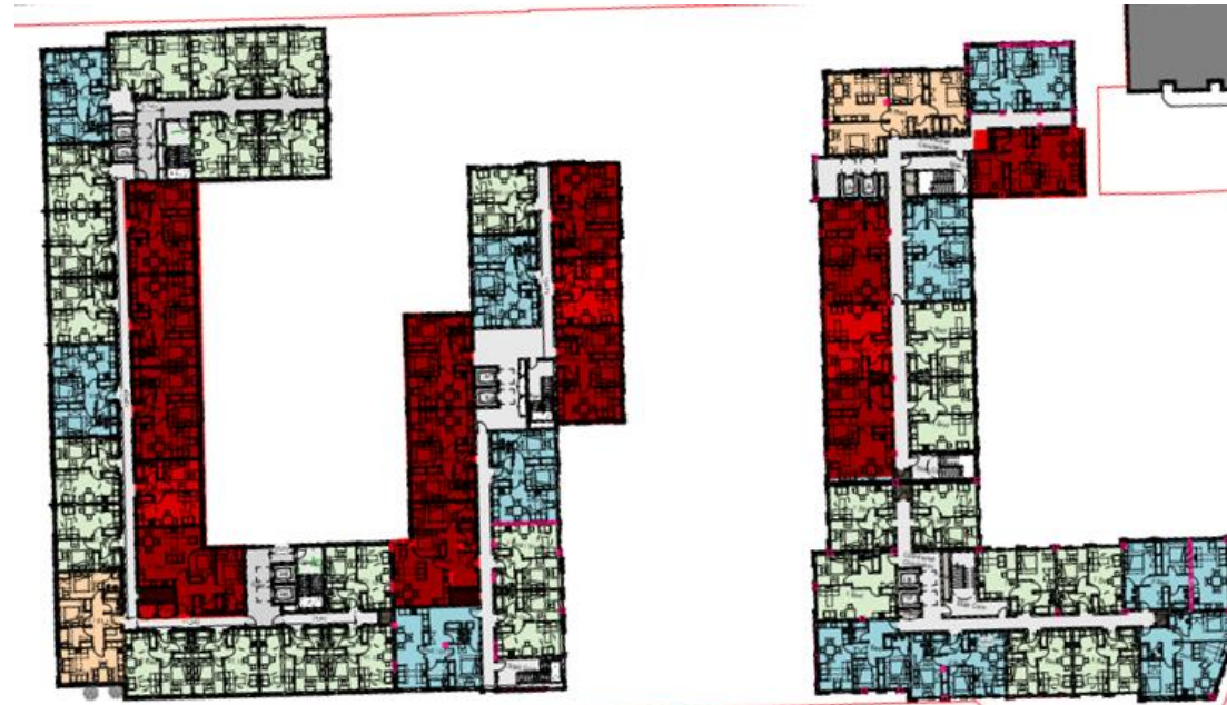
Figure 18 - Dwellings failing to meet the NSL criteria (shown in red)
