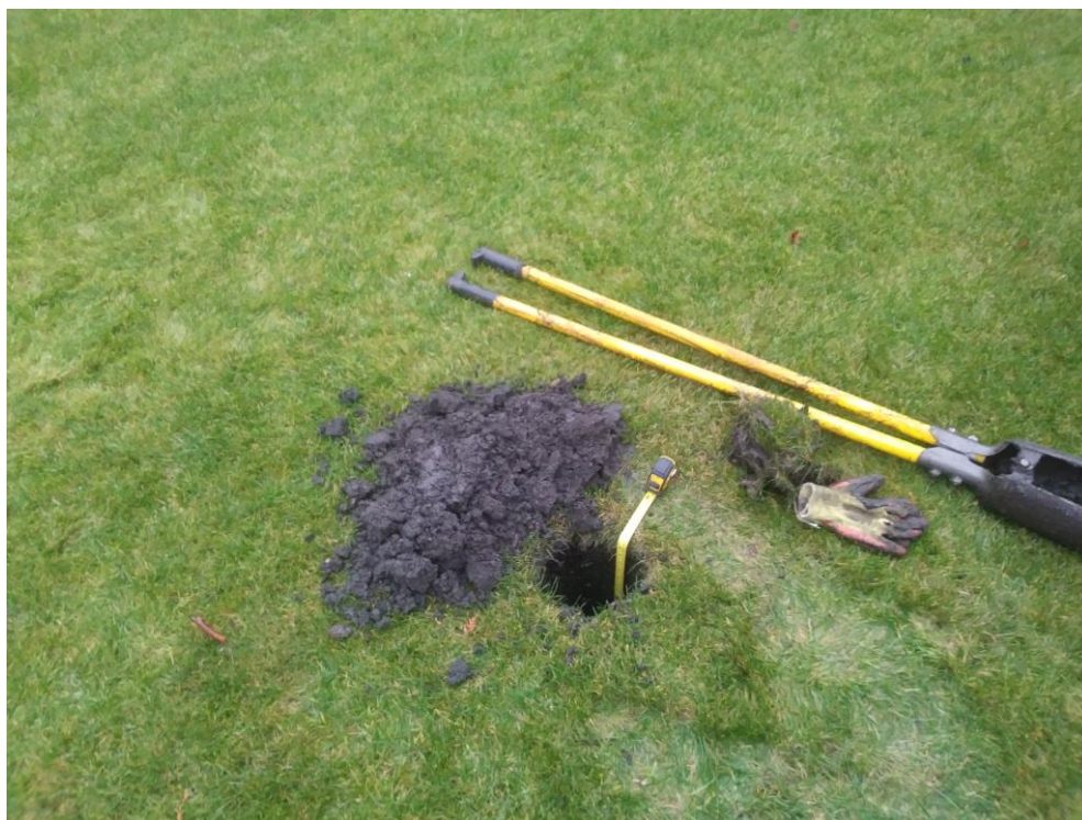
Photo 6: P3 – 490mm topsoil
