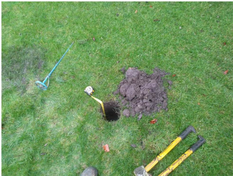
Photo 2: P1 – 380mm topsoil
