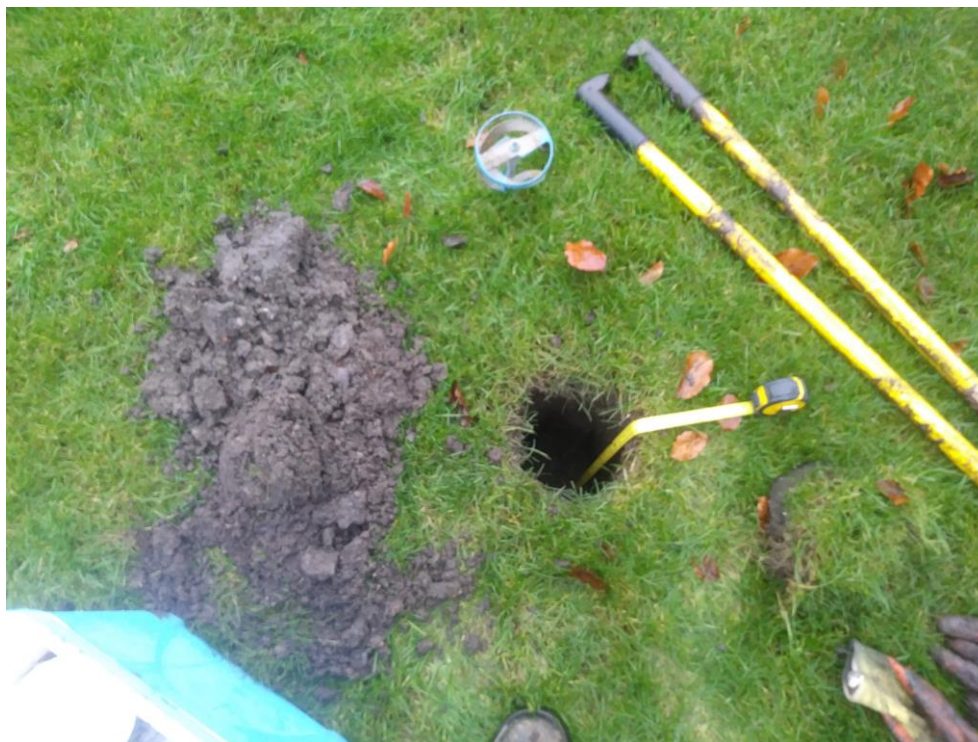
Photo 4: P2 – 400mm topsoil
