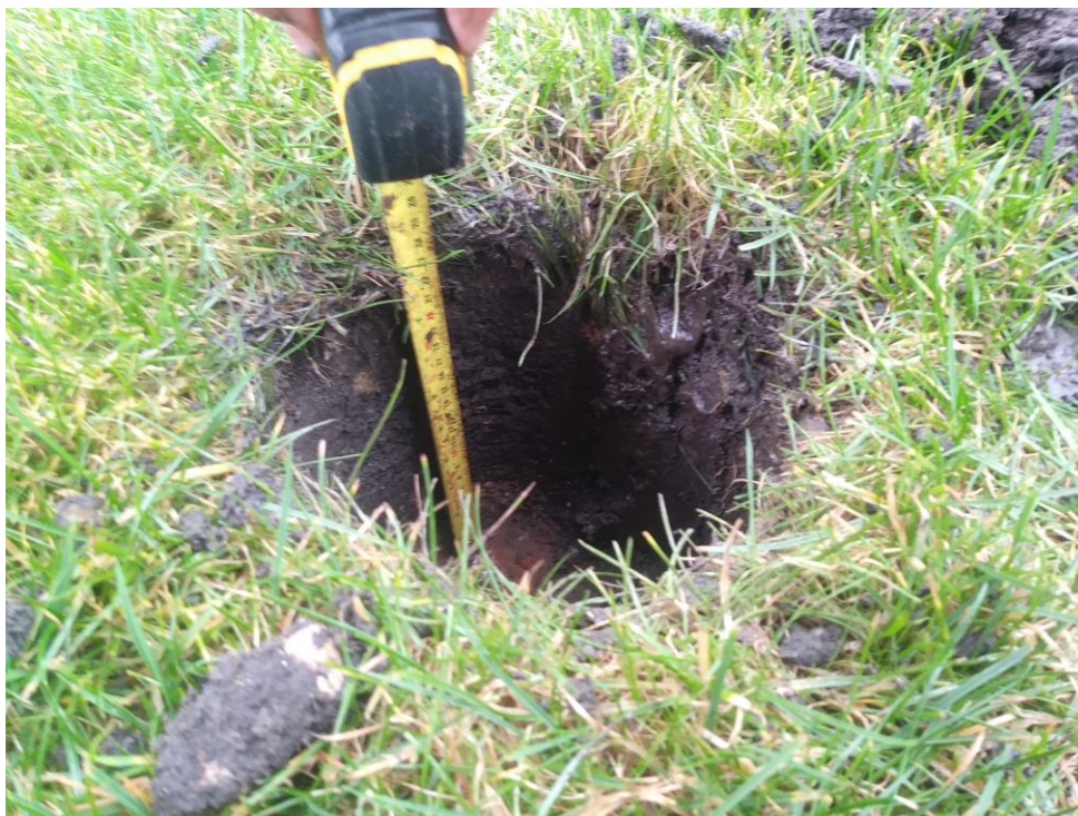
Photo 10: P5 – 250mm topsoil
