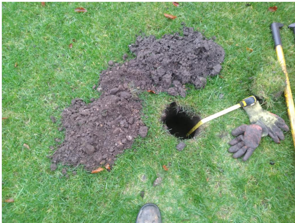
Photo 12: P6 – 150mm topsoil
