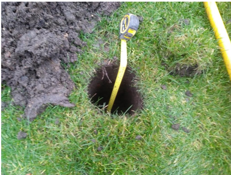
Photo 8: P4 – 450mm topsoil
