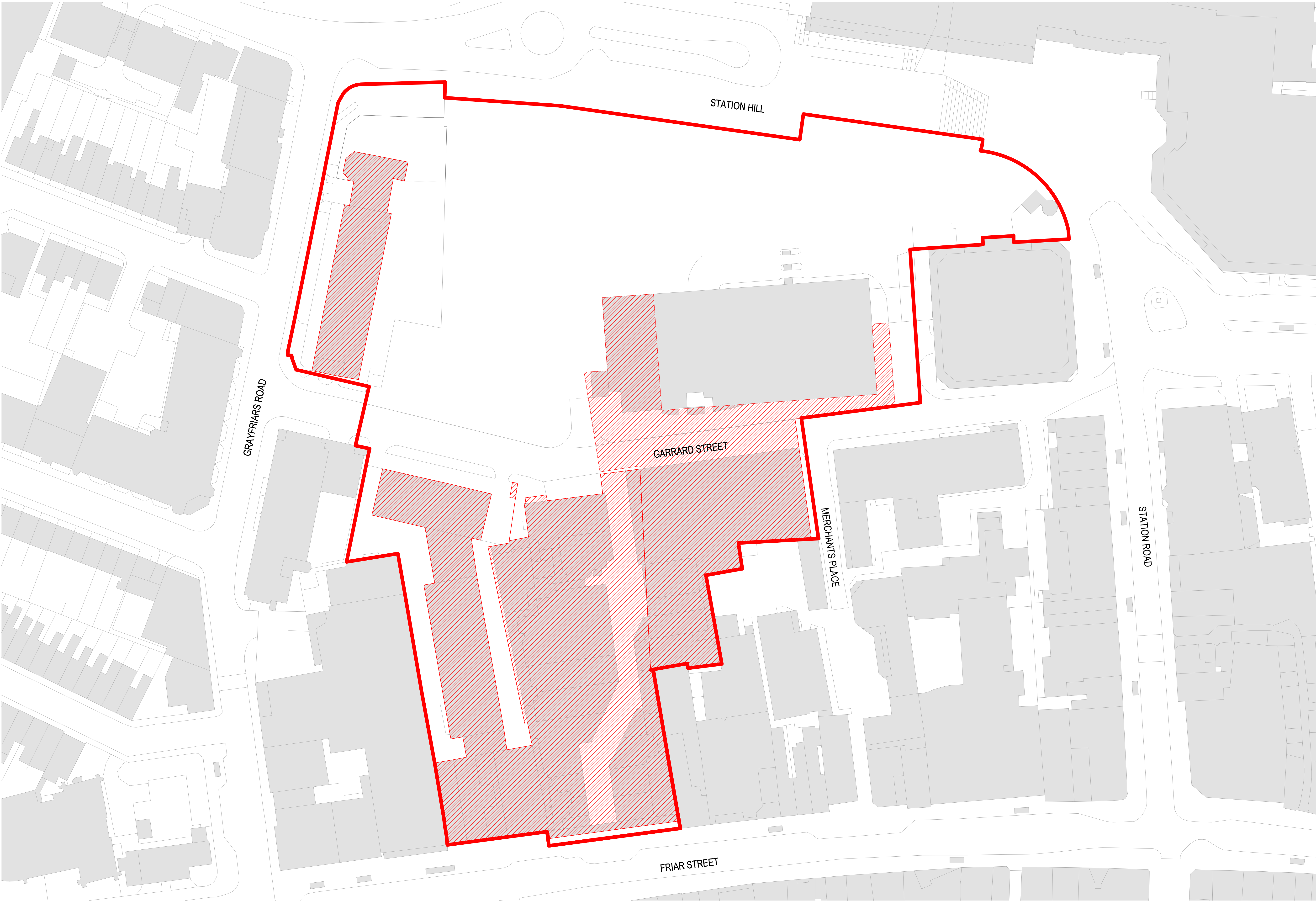
Parameter Plan_Block E - Demoliton and Retained Buildings 1 : 500
