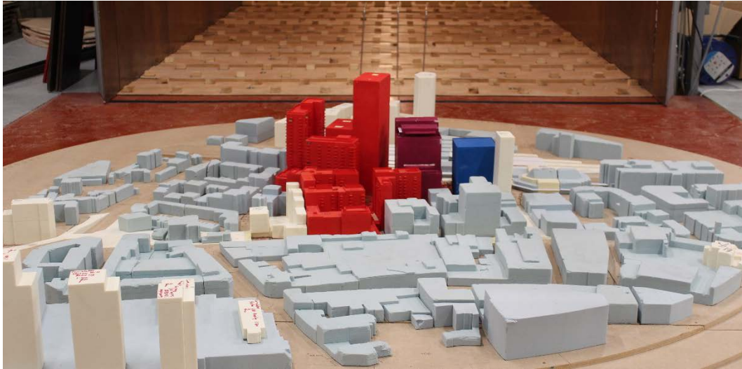
Figure 47: Development Option 3 with Landscaping, Wind Mitigation and the Cumulative Surrounding Buildings – View in the Wind Tunnel (from the south)
