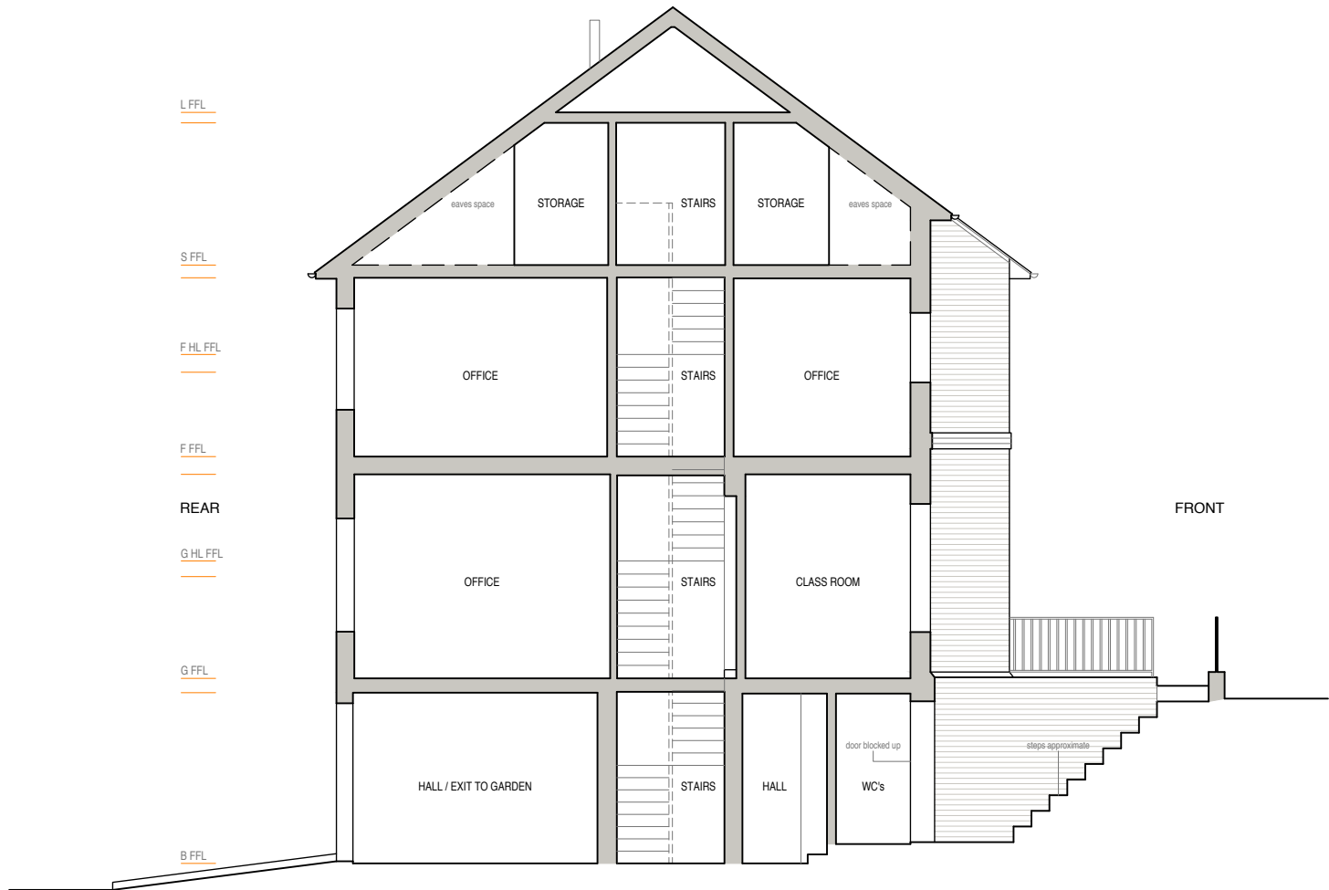
SIDE SECTION / ELEVATION (A) (WEST)
