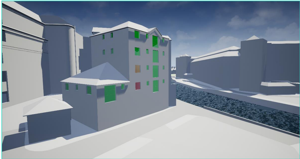
Extract 08: Window Plan Illustrating NSL Compliance (Green) & Derogations (Orange/Red)
