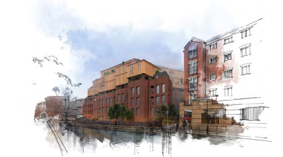
The final and chosen option which is more articulated with less height that works well with the surrounding area. The proposed uses brick for the base part with aluminium cladding for the upper parts.
