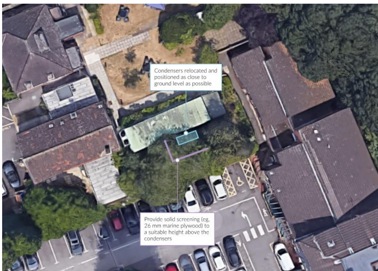
Figure 2 Recommended relocation of plant
