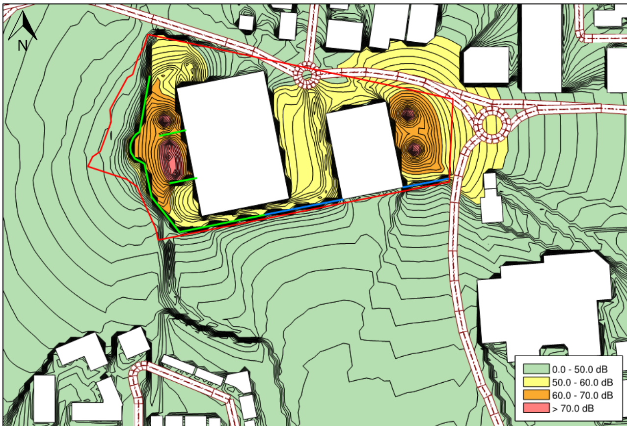
Figure 6.2 Worst-case Night-time Operational Noise Contour Plot L_{Aeq,15mins} with 4.0m high barriers including indicative extension (Grid Height 4.0m)
