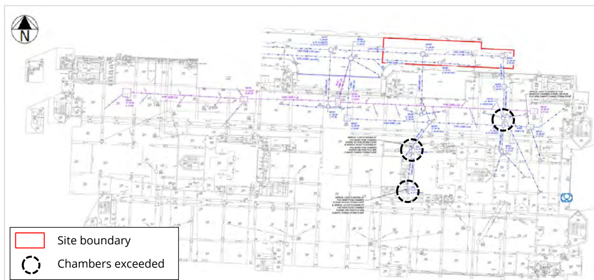
Figure 5: Drainage layout and areas of chamber exceedance
