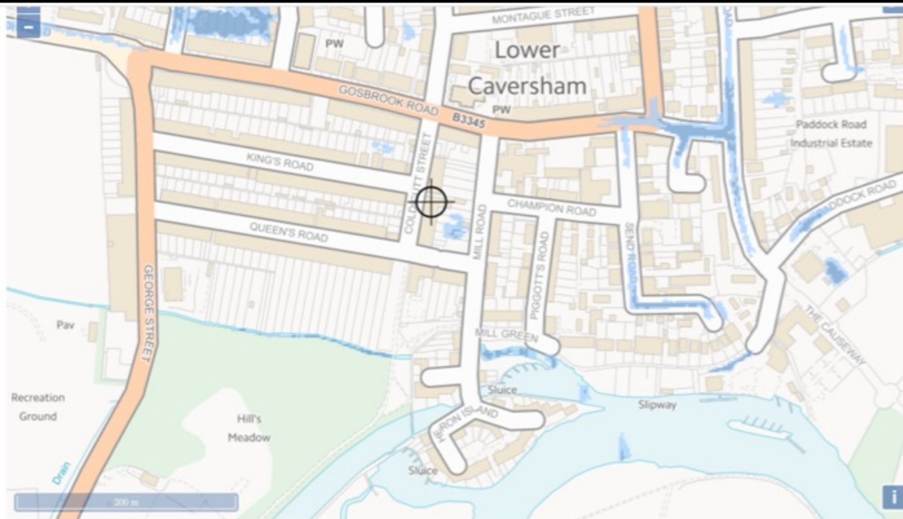
Figure 6 Environment Agency's Surface Water Flood Depth Map
