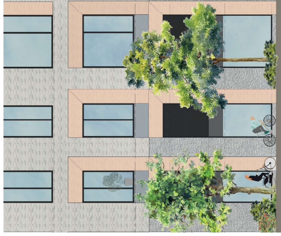
Bay study showing use of different colours from base to middle and contrasting to floor as a framing detail
