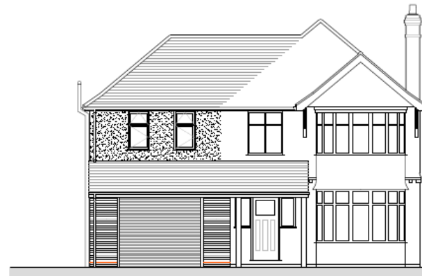
PROPOSED NORTH ELEVATION SCALE 1 : 100
