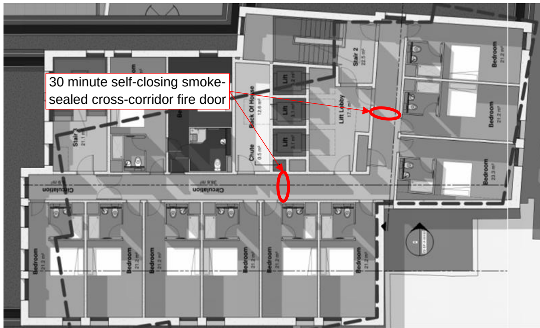
Figure 5 – Provision of cross-corridor doors at Level 07
