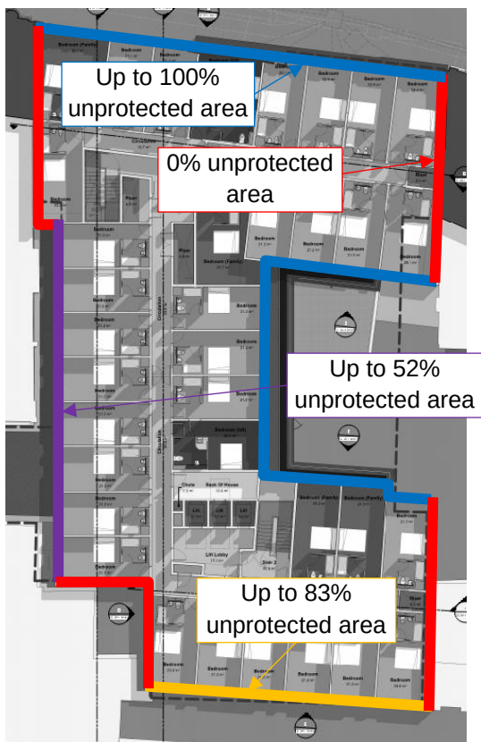
Figure 10 – Protection to the external walls at Levels 02-03 to address external fire spread
