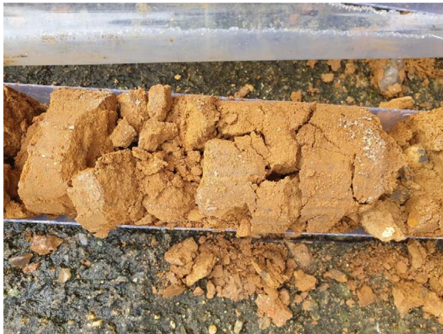
Photograph 12: Clean sands at shallow depth at BH3.
