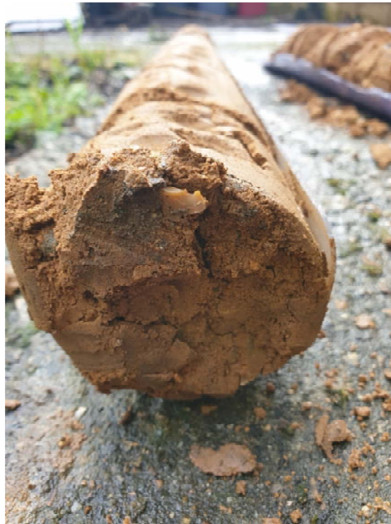
Photograph 13: Clean sands observed at base at BH3.
