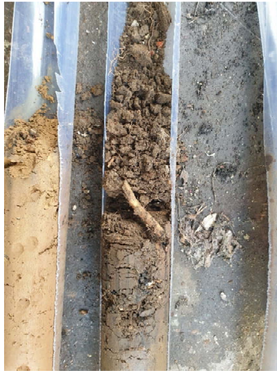
Photograph 3: A closer view of the topsoil from BH1
