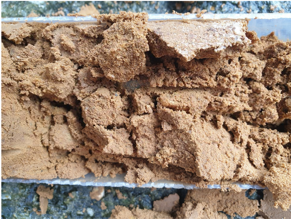
Photograph 9: Soft clean sand from Bh2 at 0.8m bgl.
