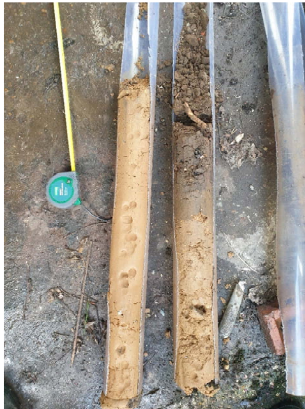
Photograph 2: A view showing the recovered soil profile from BH1 showing darker topsoils and underlying coarse sands and sandy clays.
