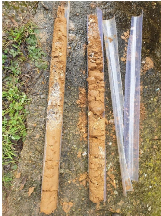
Photograph 11: Recovered soil profile from BH3.
