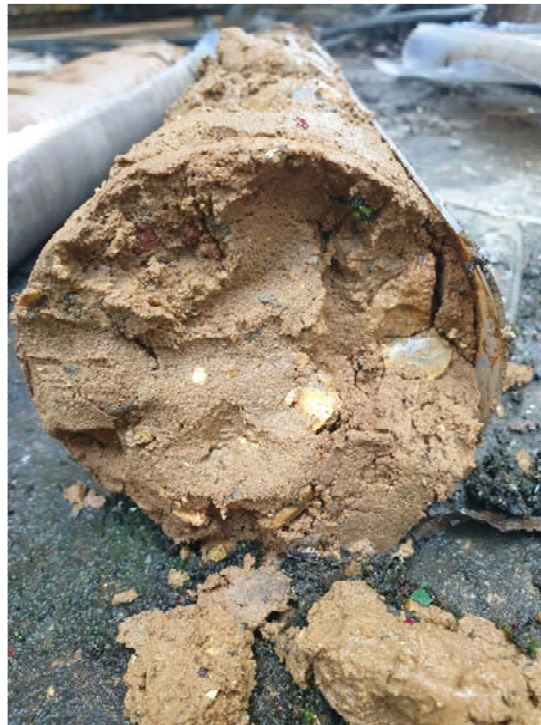
Photograph 5: A view of the end profile at 1 metre showing sands with gravel
