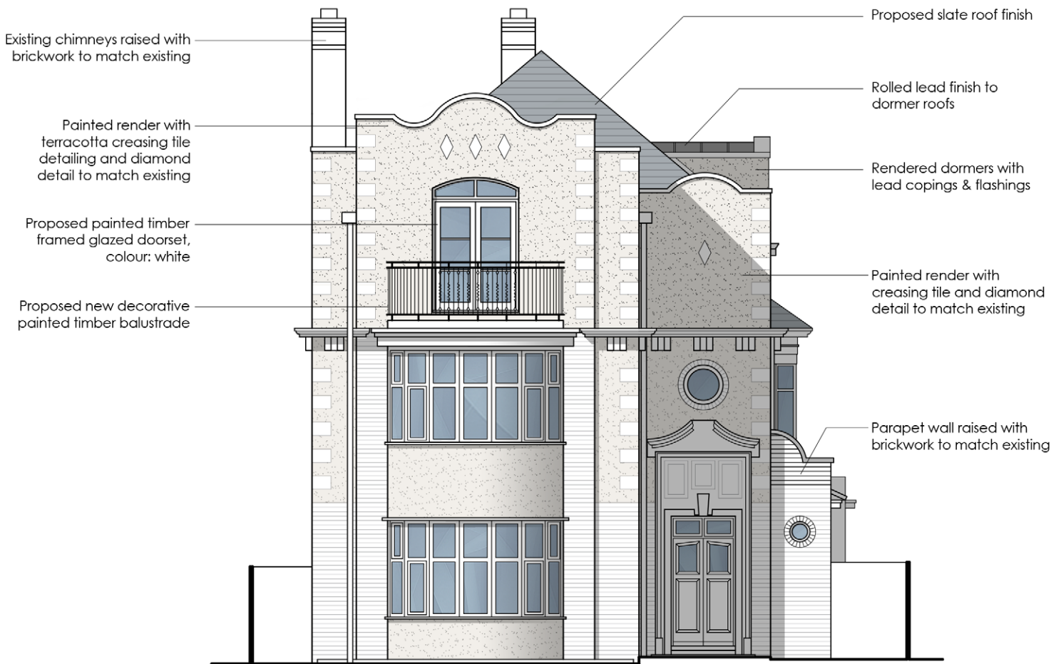
PROPOSED WEST ELEVATION (FRONT)
