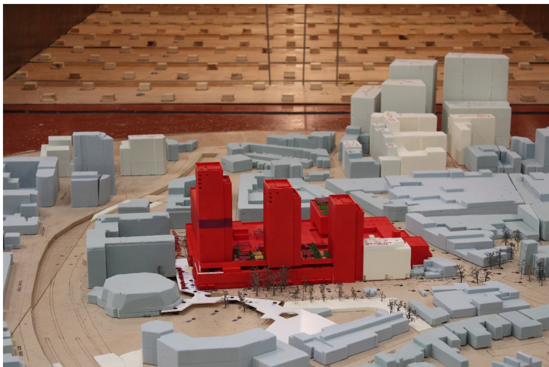
Figure 18: Configuration 2 - Proposed Development with Cumulative Surrounding Buildings, Landscaping and Mitigation Measures - View in the Wind Tunnel and Landscaping (from the south)
