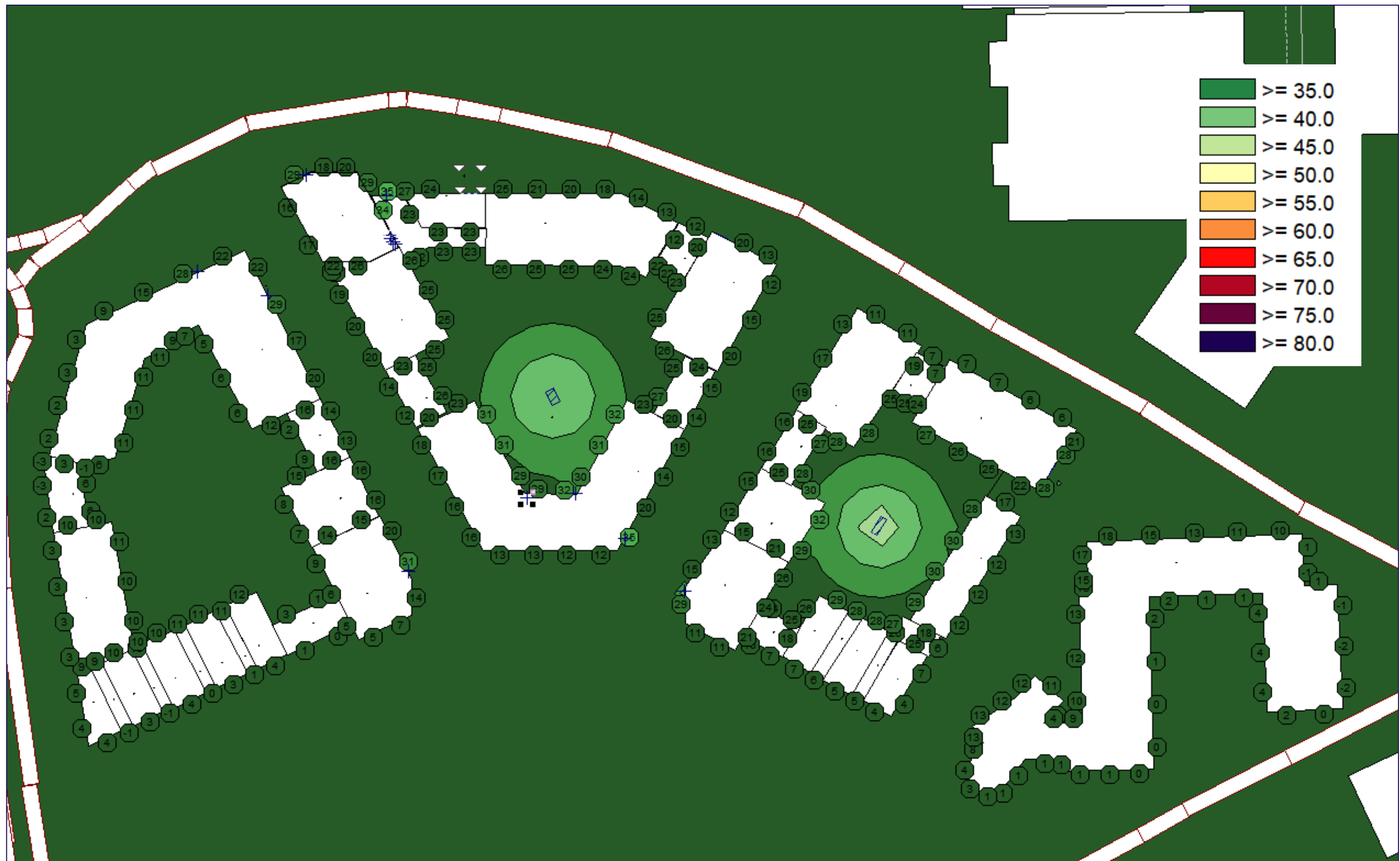
Figure 4—12 Highest calculated LAr,T noise levels 1m from the Kenavon Drive and existing NSR façades under a cumulative impact assessment scenario with all plant items / compounds operational
