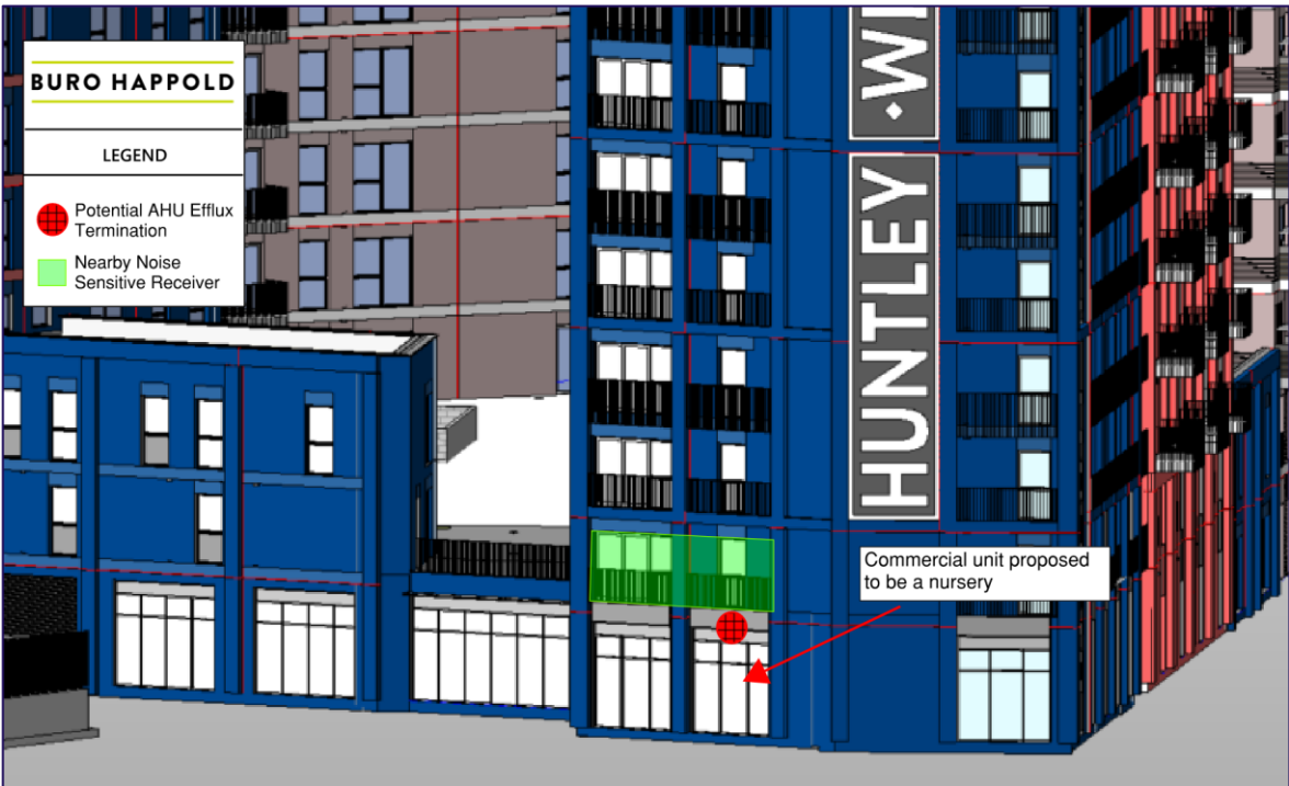
Figure 4—11 3D screenshot of Revit commercial nursery unit and the potential location of AHU plant near sensitive Kenavon Drive receivers (Source Project Revit Model: O446-AA5990C-M-ZZ-A-MIDDLE.rvt, Issued 20/08/2020)
