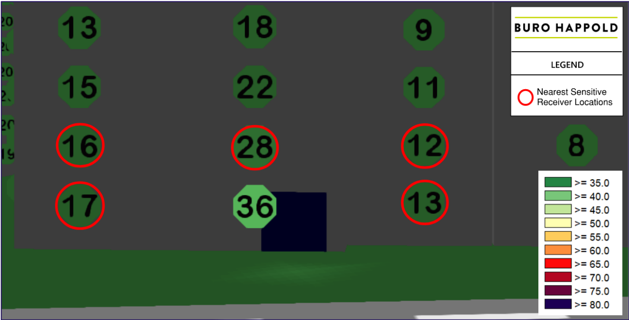
Figure 4—5 Highest calculated L_{A,T} noise levels 1m from the Kenavon Drive façade with attenuated middle block substation noise levels
