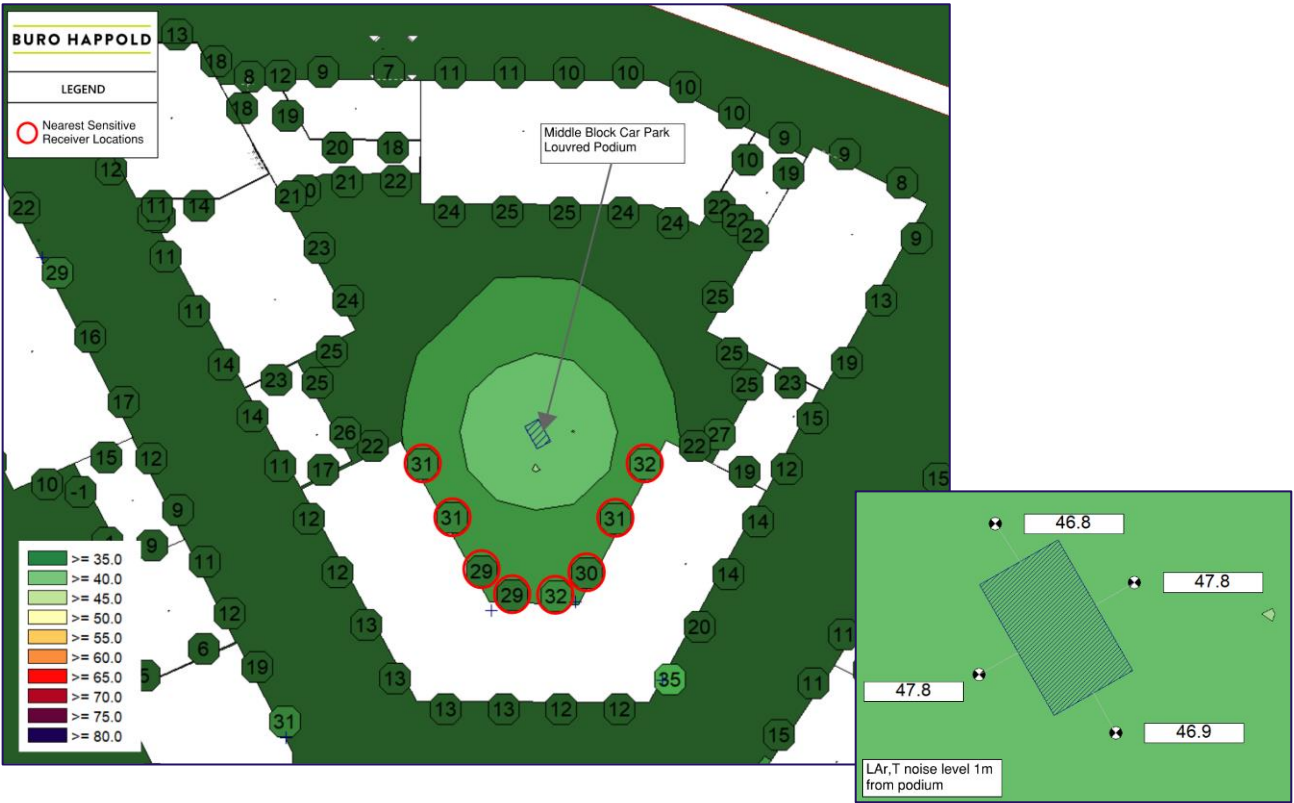
Figure 4—8 Highest calculated LAr,T noise levels 1m from the Middle Block Kenavon Drive NSR façades (left) and podium vents (right) – implemented acoustic attenuation elements detailed in Table 4—6.
