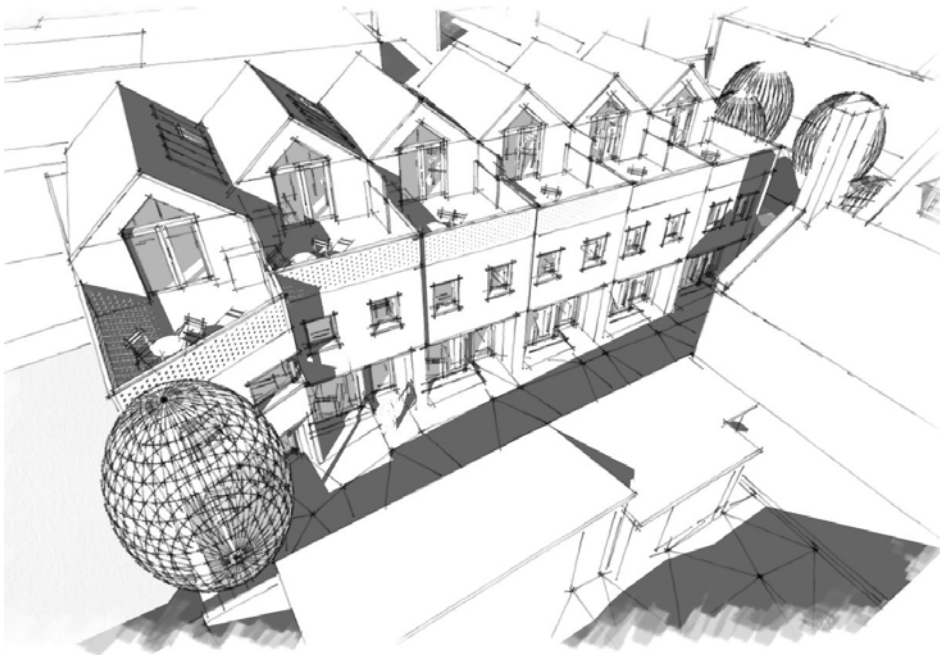
Sketch from energy report modelling solar shading and solar gains.
