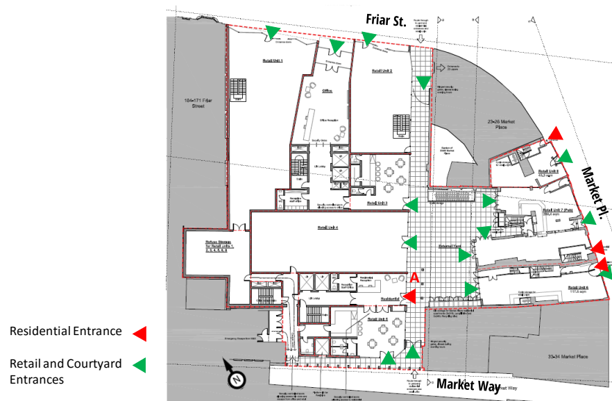
Figure 5: Ground floor plan showing the location of entrances
