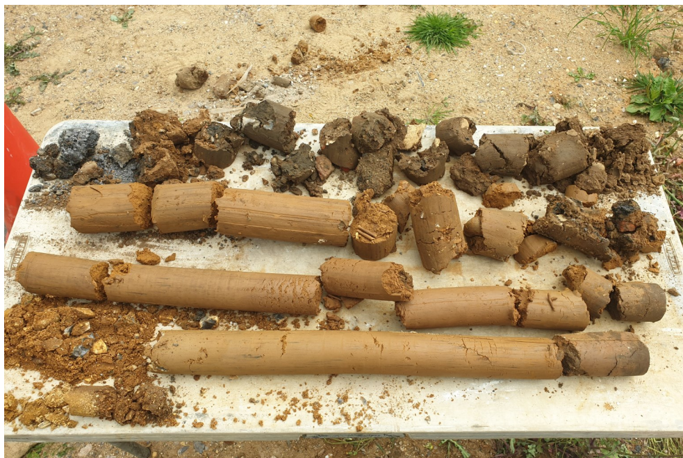
Photo of arisings from boreholes WS5
