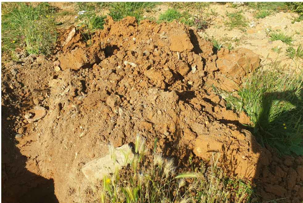
Photo of arisings from trial pit SA2
