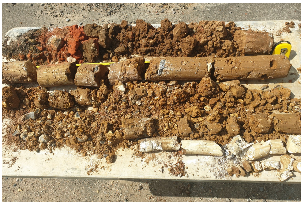
Photo of arising from boreholes WS2
