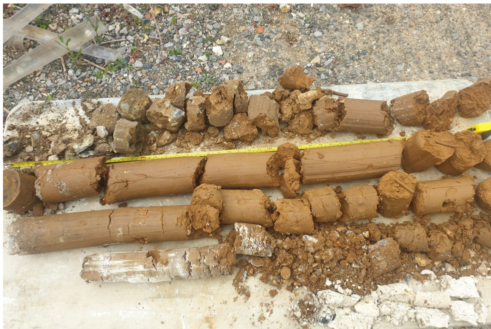
Photo of arising from boreholes WS1
