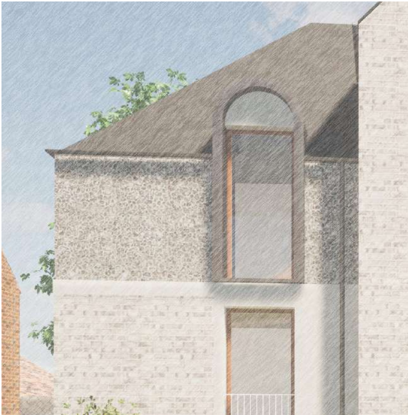
Flint paneling references the use of flint on the neighbouring Ivy Farmhouse. A cast stone stringer course separate the flint from the brick creating a crisp junction.
