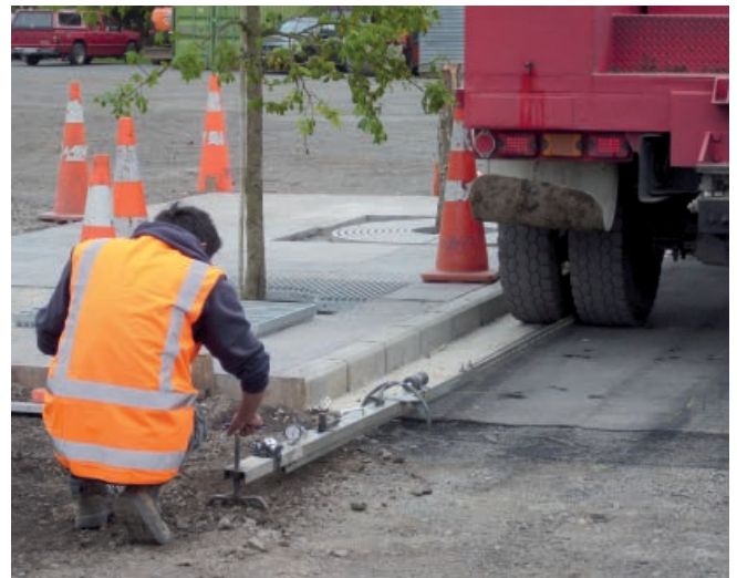
The RootCell structure underneath this pavement was subjected to 400 passes of an 8.2 tonne (9 ton) axle loading immediately adjacent to the structure and then a further 200 passes immediately above the RootCell . As expected, no adverse movement of the structure was detected
