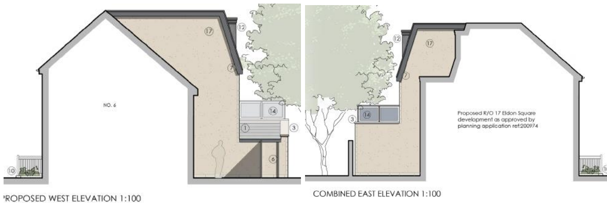
Now proposed side elevations showing the now proposed limestone colour sand and cement render finish.
