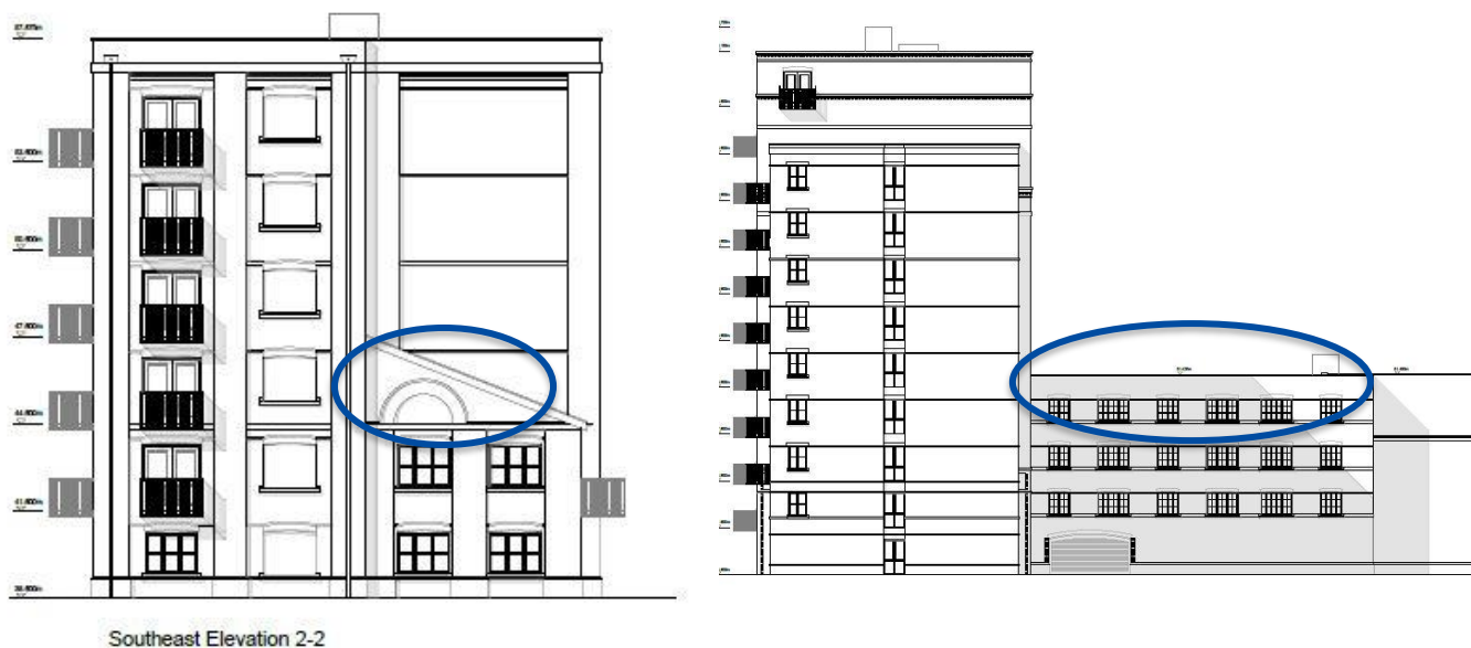
Figure 4 – Lower Roofspaces for Blocks A (left) and B (right)
