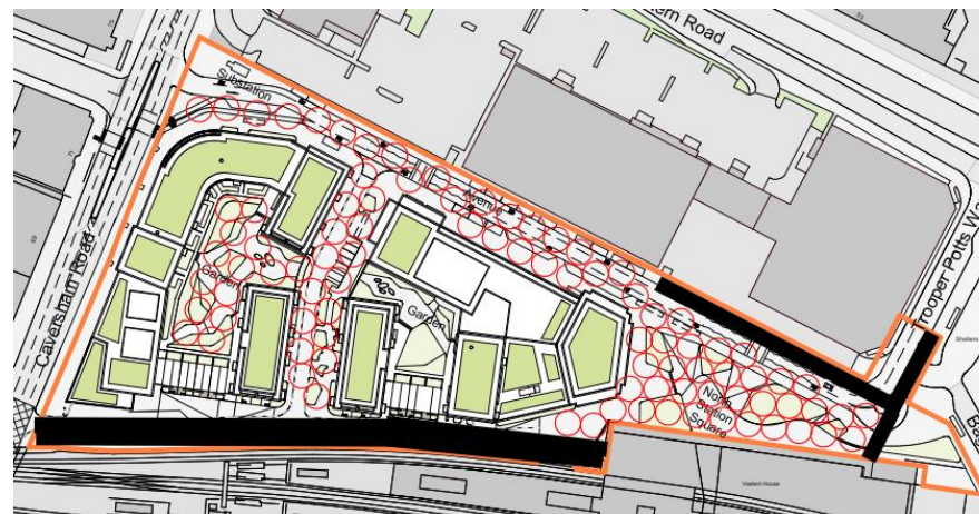
Figure 10: Analysis of available space for borehole field
