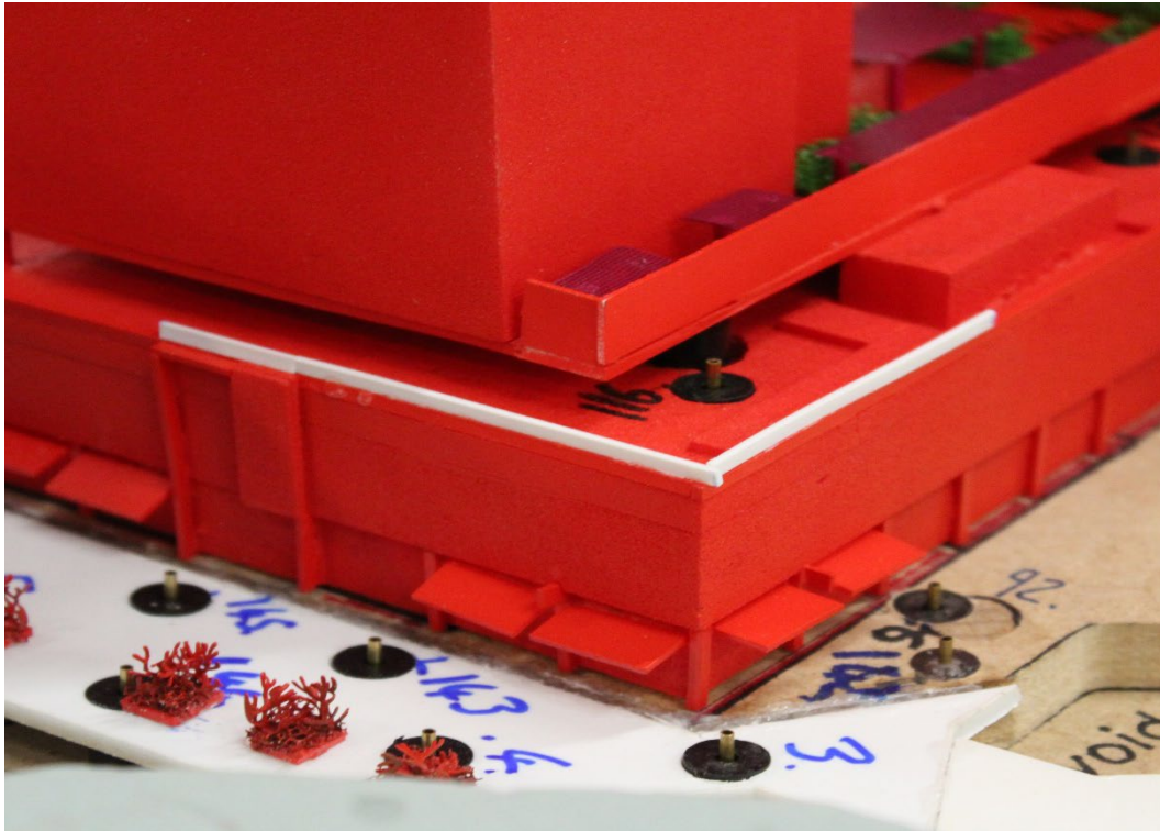
Figure 20: An increase in the height on the balustrade on the south-western corner, from 1m to 2
