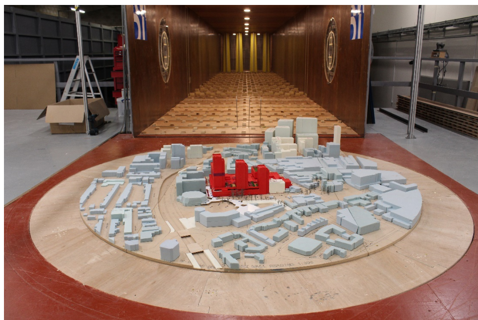
Figure 2: Image of the Proposed Development with Cumulative Surrounding Buildings, Landscaping and Mitigation Measures. (View in the wind tunnel from south)
