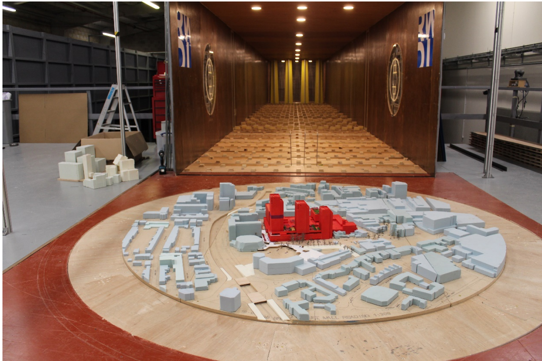
Figure 15: Configuration 1 - Proposed Development with Existing Surrounding Buildings, Landscaping and Mitigation Measures - View in the Wind Tunnel (from the south)
