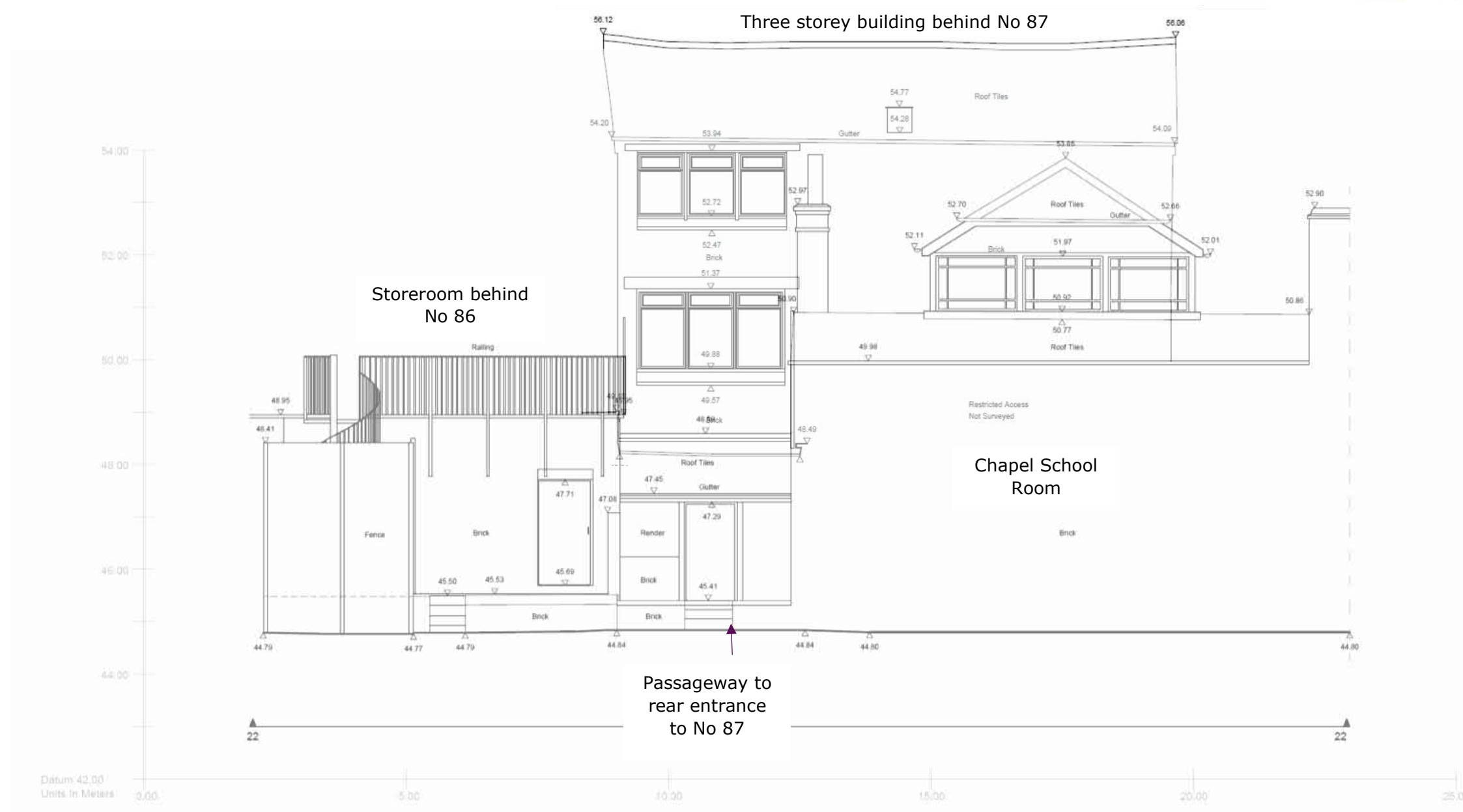
Figure 15: Rear elevation showing the rear of the storeroom behind No 86 and the three storey structure behind No 87 and later corridor between the storeroom and former school room for the chapel that was built on the former graveyard (Elevation Surveyed and drawn by MK BIM Solutions and amalgamated for this illustration)
