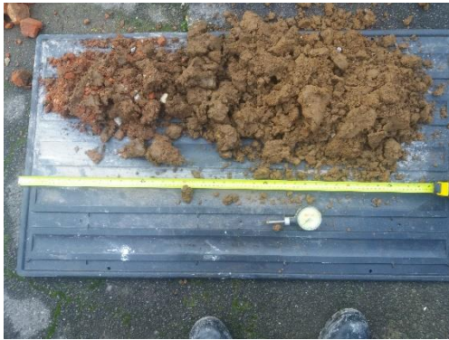
Photograph 7 - Looking down at near surface material arisings within WLS2 [surface to 1m bgl].
