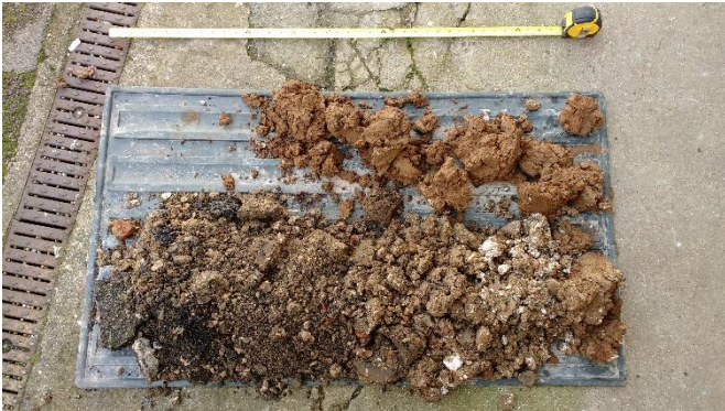
Photograph 9 - Looking down at near surface material arisings within WLS3 [surface to 1m bgl].
