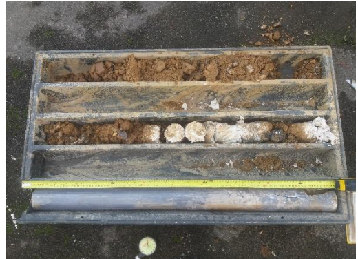
Photograph 8 - Looking down at material arisings from WLS2 [1m - 3.45m bgl].
