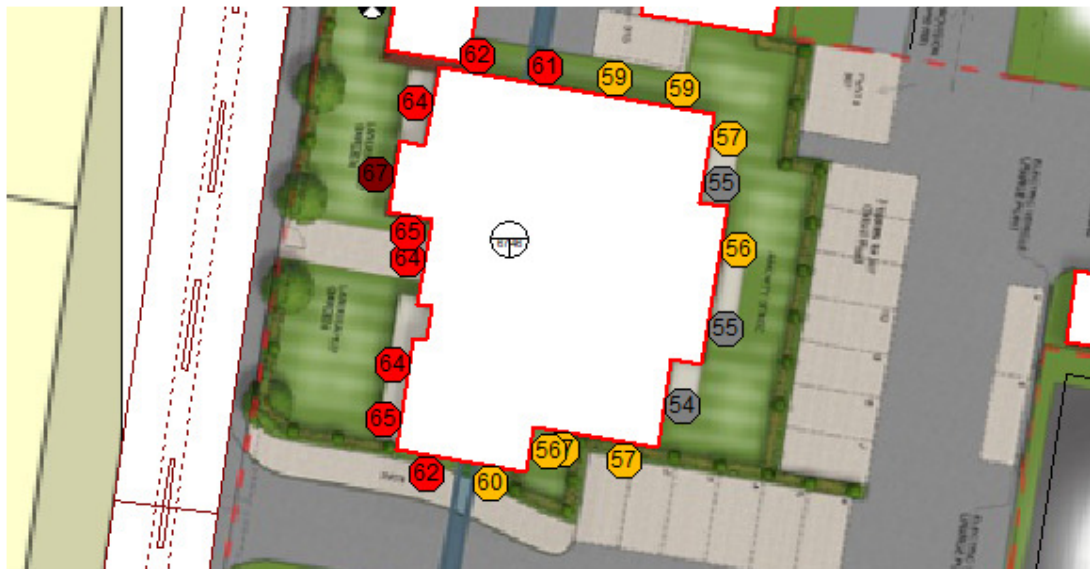
Figure 4: Predicted with-scheme Façade L_{Aeq,16h} Noise Levels day
