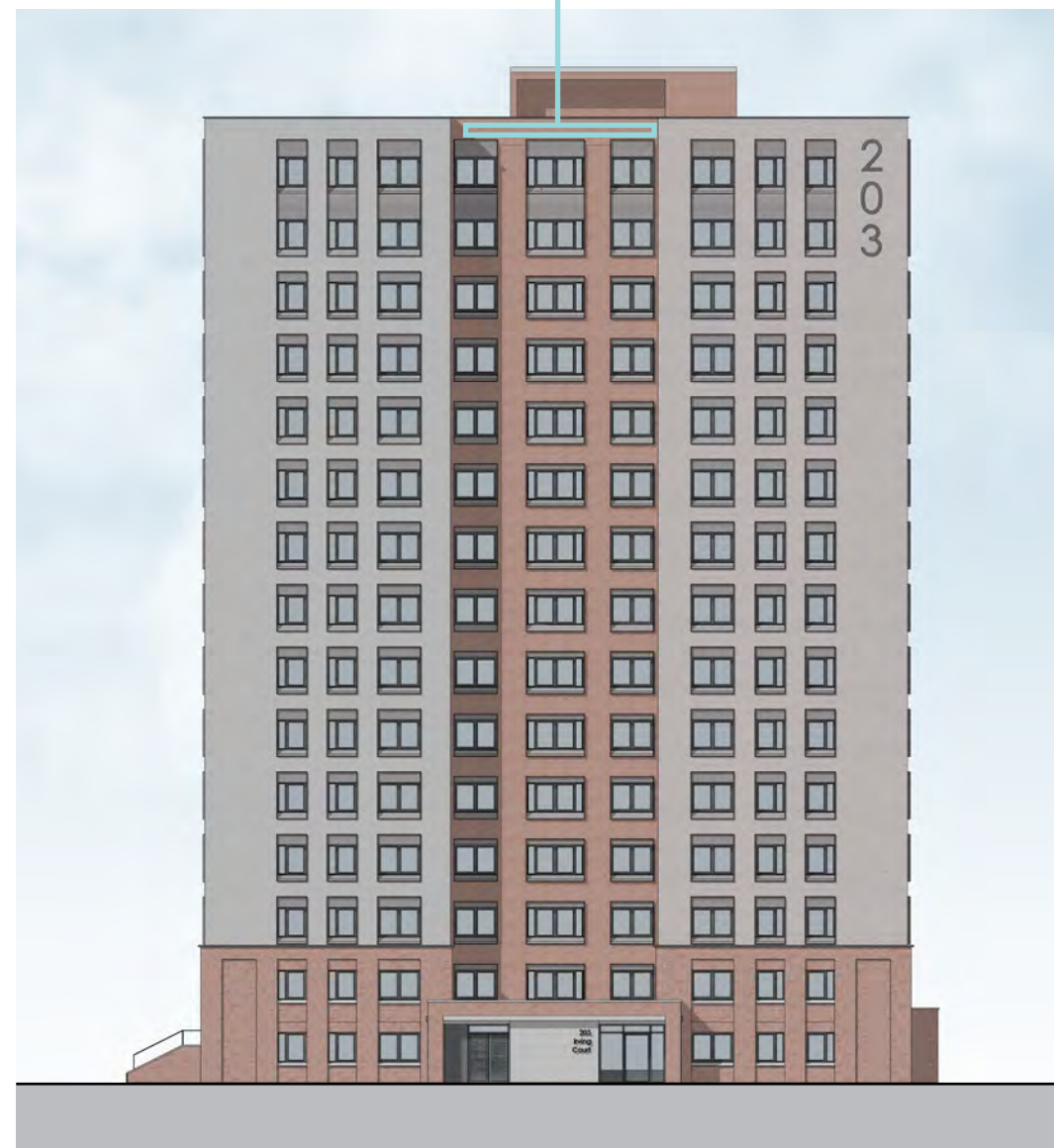
Typical Front Elevation - Swift Box Locations
