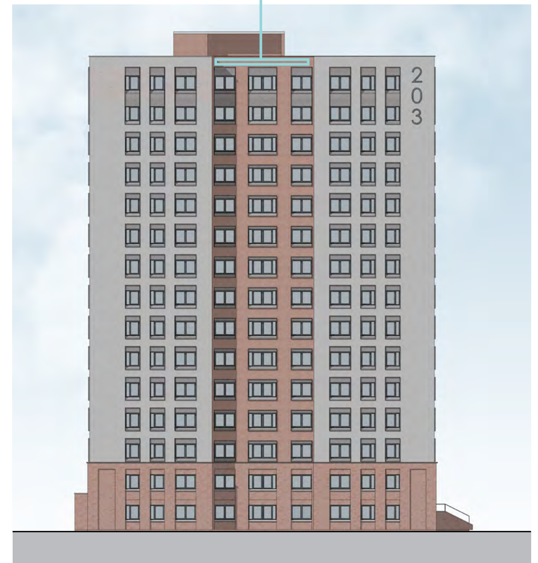
Typical Rear Elevation - Swift Box Locations
