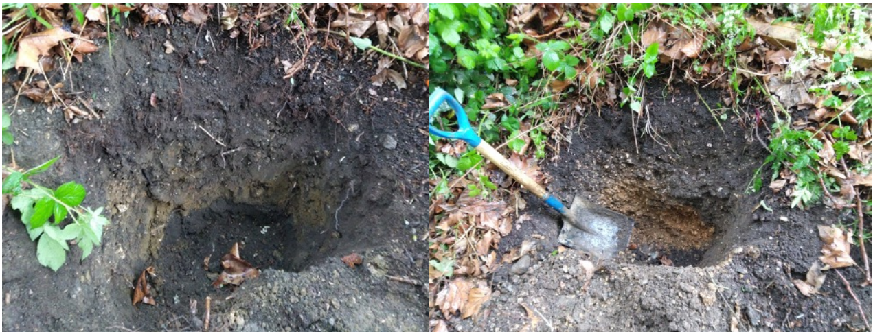
Photo 6 and 7: showing the trial pits excavated in the CEZ of T1. Photo 6 was excavated approximately 3m south of the stem of T1 and to a depth of circa 400mm. Photo 7 was excavated approximately 1m north of the existing retaining wall to a depth of circa 600mm on the alignment of the platform required for machine access (similar location to that shown in photo 5).
