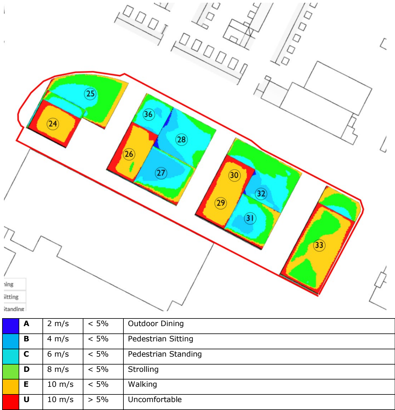
Figure 9.7: Configuration 2 – Roof Level (Pedestrian Comfort)
