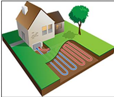
Horizontal Loop System
