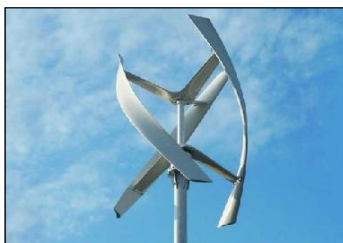
Vertical Wind Turbine
