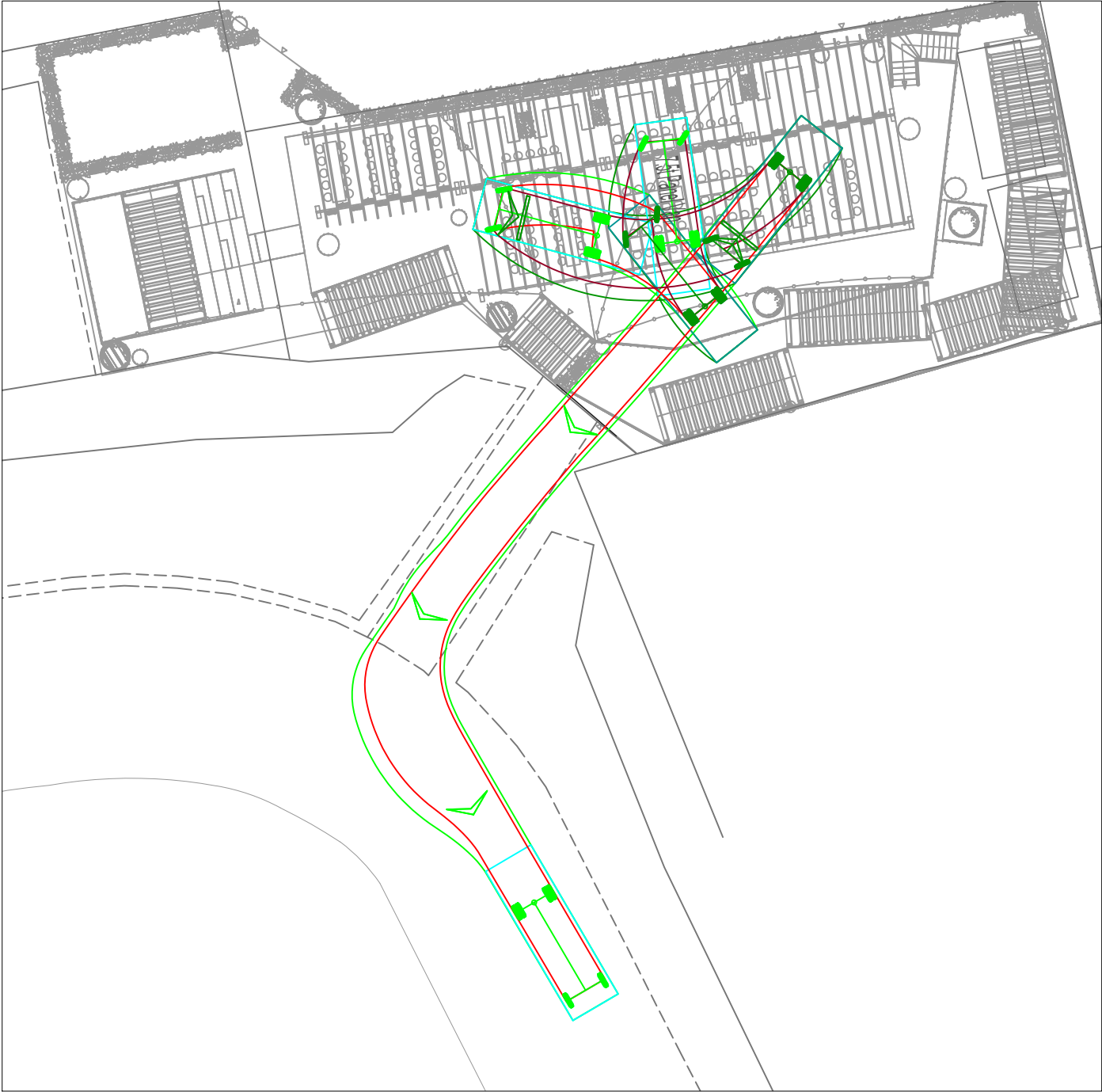
Swept Path Analysis of a 7.2m Delivery Van Performing a 4 Point Turn and Exiting Site Access
