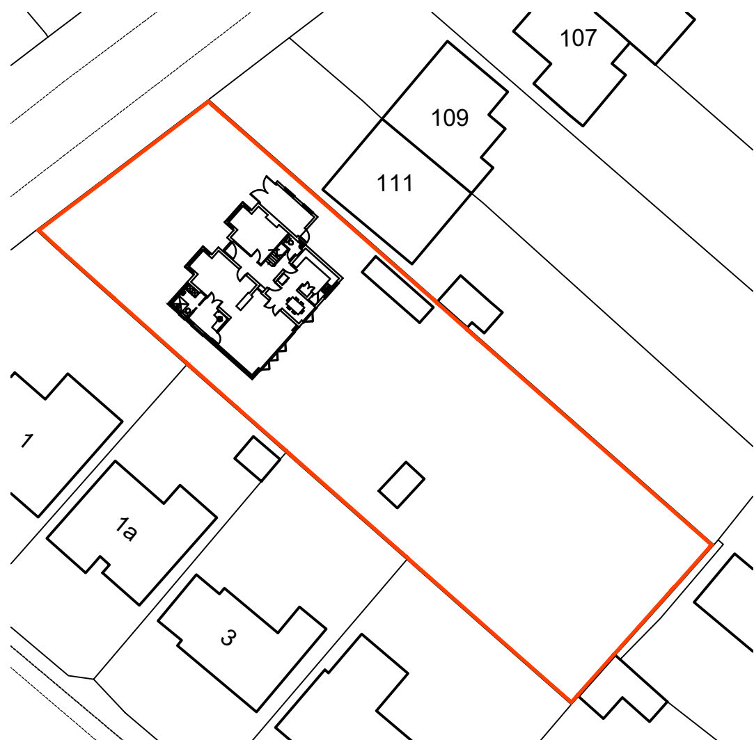
Site/Block Plan (scale 1:500)
