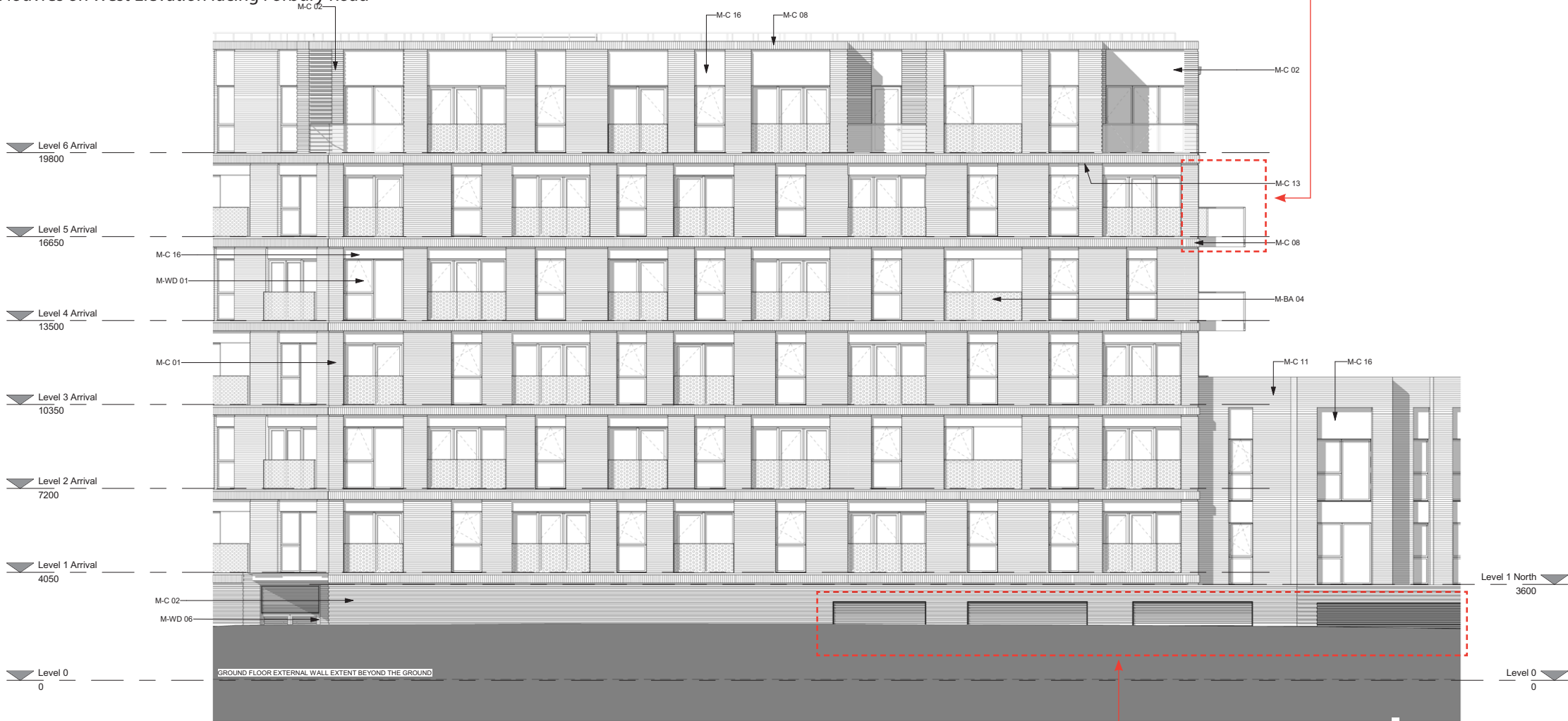
High-level ventilation louvres added to the West Elevation to support the "mixed ventilation" system using a combination of exterior openings, a mechanical extract system and impulse fans.
