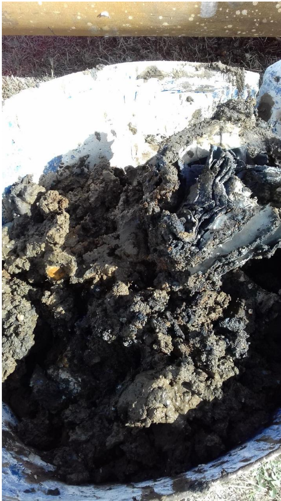
PLATE 16: BH03 LANDFILL MATERIAL
