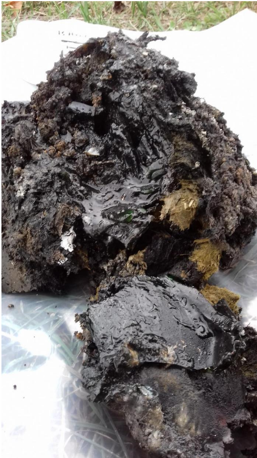
PLATE 12: BH01 SLUDGE MATERIAL FROM 1.50MBGL
